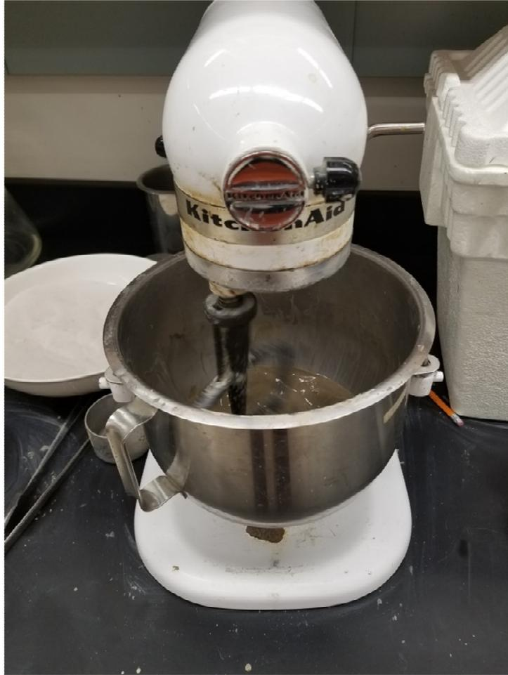
***Figure 3- 2: Using a stand Mixer to Blend the Clay and Saline Solution for Resedimentation***
