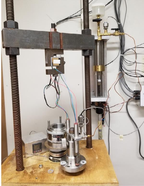
**Figure 3- 11: Photograph of Typical Tufts Automated CRS Testing Apparatus**
