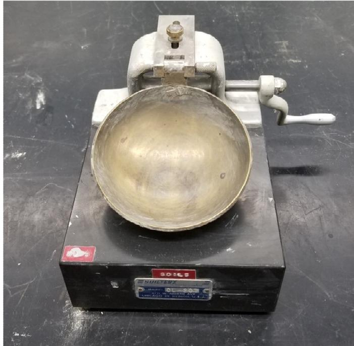
**Figure 3- 13: Cassagrande Cup used for Liquid Limit Testing**
