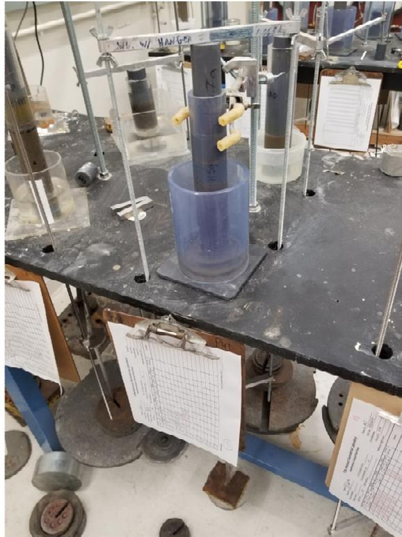
**Figure 3- 5: Typical Consolidometer used for Resedimentation**
