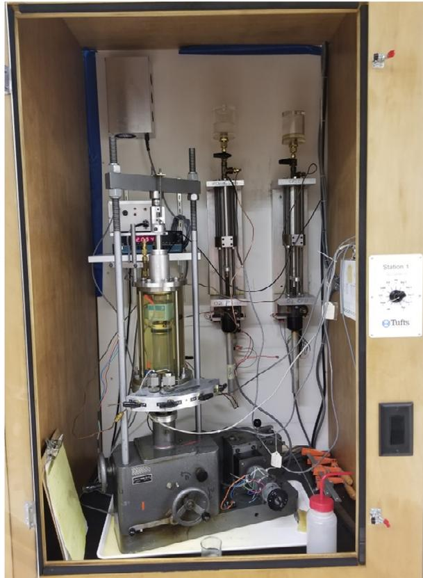
**Figure 3- 9: Photograph of Typical Tufts Automated Triaxial Testing Apparatus**
