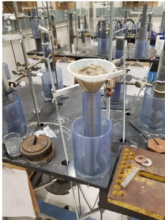
**Figure 3- 4: Tremieing the Clay Slurry into a Consolidometer**
