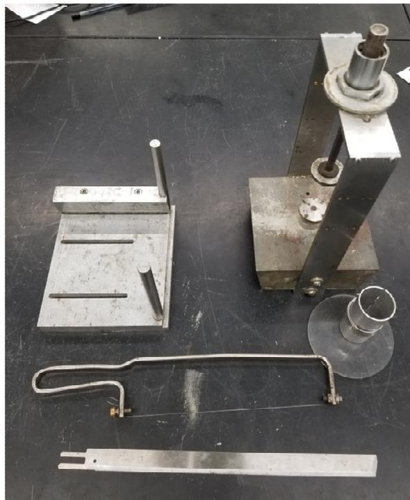
**Figure 3- 6: Triaxial Test Specimen Trimming Equipment**
