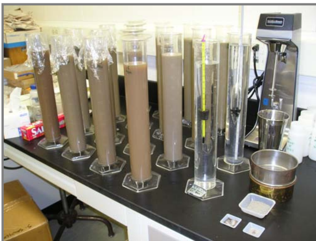
Figure 3: Several hydrometer analyses performed at the same time. Image is from set up at Penn State showing malt mixer, sieve, hydrometer, thermometer and materials on right hand side.
