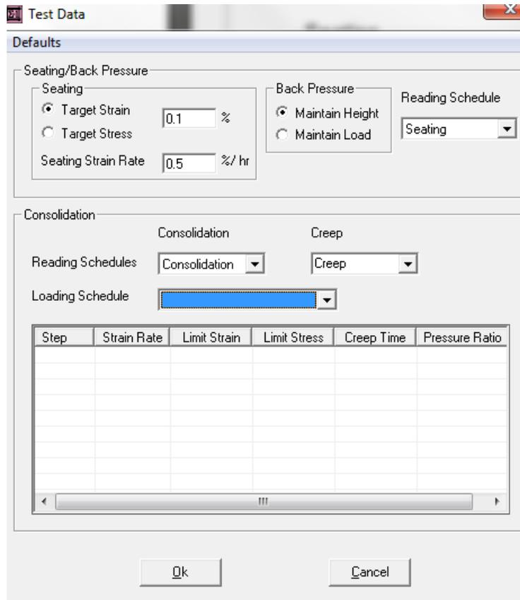
[ ] in the test data window, select a **loading schedule** appropriate for your test specimen, testing plan, and apparatus configuration. If an appropriate loading schedule is not already set up, you will need to create one yourself (*Appendix to be written*).
