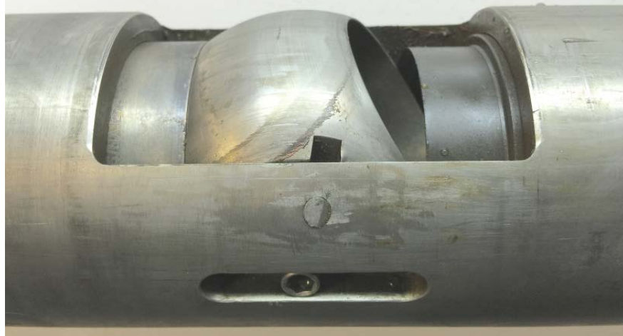
Figure 2.3.3 Photo showing the half-open ball valve sealing mechanism in the PCTB.
