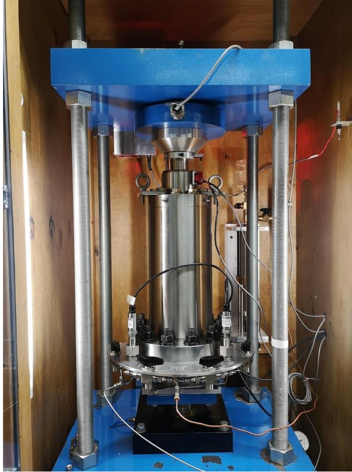
Fig. 2: High pressure triaxial cell - capable of withstanding up to 100 MPa cell pressure
