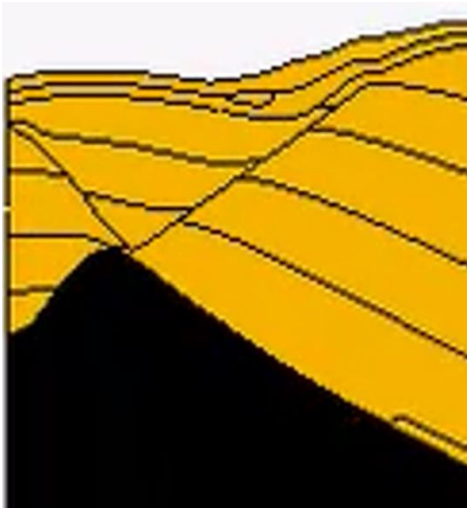
Fig 1: The salt wall rising and faulting its roof. Salt is black and sediments are yellow. (a) Entire model. (b) Salt-wall roof (Box A in a).
