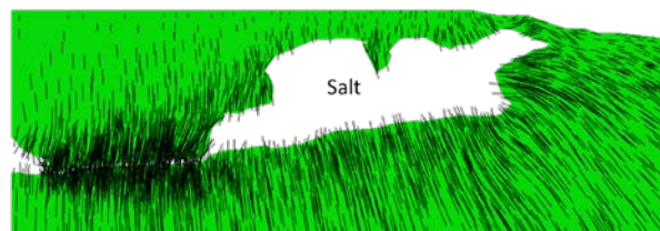
Fig. 1: Orientation of maximum principal stress predicted by geomechanical model in a salt basin, Mad Dog field, Gulf of Mexico. Stresses are strongly perturbed particularly in front of salt due to large lateral thrust from salt and updip sediments.
