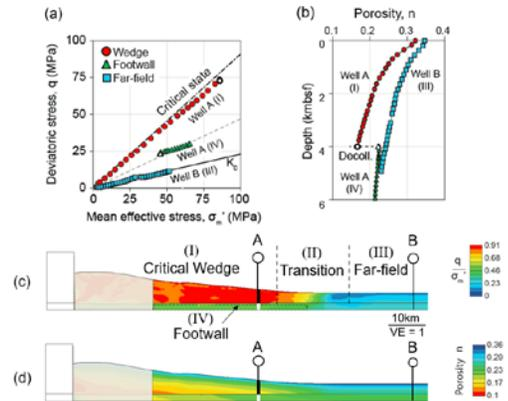
**Fig 1:** Stress and compression distribution in a fold-and-thrust belt.
