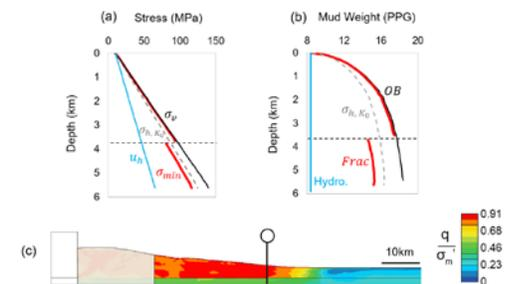
**Fig 2:** Stress and fracture gradient across decollement
