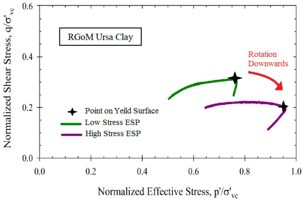
**Fig 2:** Shift in Yield Surface for Resedimented Gulf of Mexico Clay. A test procedure carried out at high is stress is compared to one carried out at low stress. The point on the yield surface has moved significantly. It appears that the yield surface is rotating downwards with increase in stress level.
