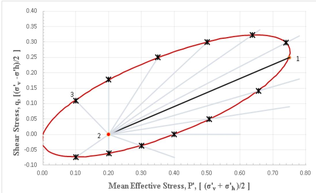
**Fig 1:** Probing with both drained and un-drained triaxial tests to identify the yield surface.
