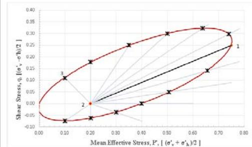
**Fig 1:** Probing with both drained and un-drained triaxial tests to identify the yield surface.
