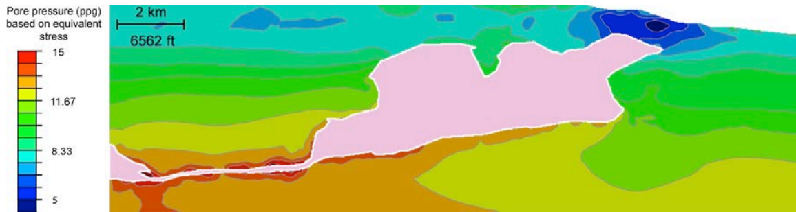
Figure 1: Predicted pore pressure at the Mad Dog field based on equivalent effective stress; the prediction accounts for the contribution of both total mean and shear stresses to overpressure.
