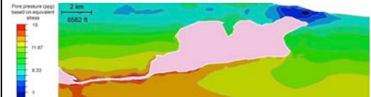
Figure 1: Predicted pore pressure at the Mad Dog field based on equivalent effective stress; the prediction accounts for the contribution of both total mean and shear stresses to overpressure.
