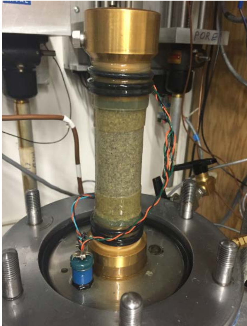
Fig. 1: Wave velocity measurement setup on triaxial test specimen.
