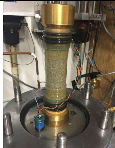
Fig 1: Wave velocity measurement setup on triaxial test specimen.
