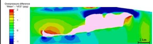
**Figure 2:** Difference in pore-pressure prediction between proposed approach, based on mean effective stress, and traditional approach, based on vertical effective stress. The traditional approach cannot account for the lateral stress loading from the salt, and hence underpredicts pore pressures near salt.
