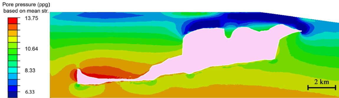
**Figure 1:** Pore pressure prediction near Mad Dog salt, based on velocity measurements coupled with static geomechanical modeling. The geomechanical model provides values for the mean stress around salt; hence the approach incorporates the lateral load from the salt in the pressure prediction.
