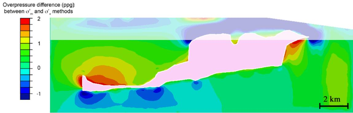
**Figure 2:** Difference in pore-pressure prediction between proposed approach, based on mean effective stress, and traditional approach, based on vertical effective stress. The traditional approach cannot account for the lateral stress loading from the salt, and hence underpredicts pore pressures near salt.
