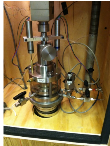
Fig 2: New radially-draining constant rate of strain (CRS) consolidometer with loading capacity up to 40 MPa developed at MIT.
