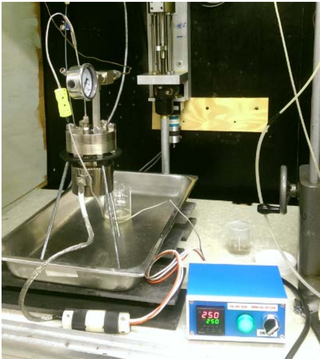
Fig. 2: Hydrothermal reactor with heating system, maximum cell pressure up to 30MPa.
