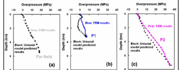
**Fig. 2:** Comparison of finite-element model (FEM) predicted overpressures with the uniaxial model predicted overpressures through far-field profile (a), near-salt P1 profile (b), and minibasin-center P2 profile (c). Profile locations are shown in Fig.1a.
