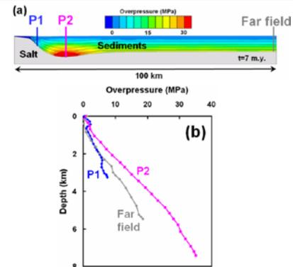
**Fig. 1:** (a) Finite-element model overpressures in sediments during sedimentation. (b) Finite-element model overpressures through different profiles across the model.
