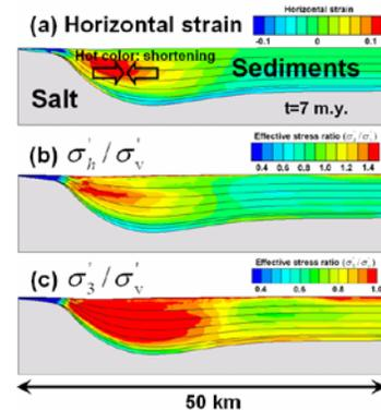
**Fig. 3:** Finite-element predicted horizontal strain (a), ratio of horizontal and vertical effective stresses (b), and ratio of minimum principal effective stress and vertical effective stress (c).
