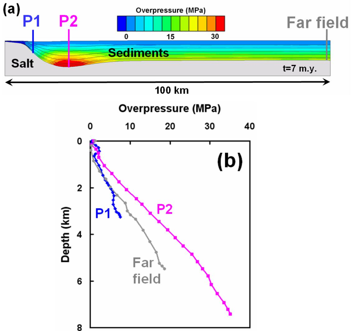
**Fig. 1:** (a) Finite-element model overpressures in sediments at 7 m.y. during sedimentation. Overpressures are concentrated at the bottom of the minibasin center. P1, P2 and far field show the locations of overpressure profiles in (b). (b) Finite-element model overpressures are different along different profiles across the minibasin. Depth on vertical axis: below sea floor.
