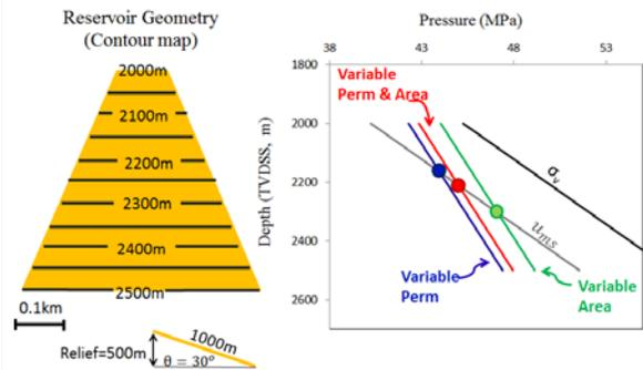
**Fig. 1:** Comparison of pressure predictions on a trapezoid-shape reservoir based on different approaches.
