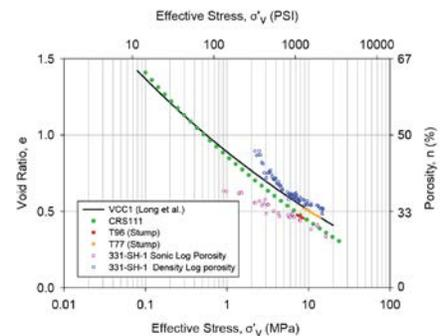
**Figure 2:** Resedimented compression curve (porosity vs. effective stress) is shown with green dotted line. Pink and blue circles record wireline estimates of in situ porosity based on sonic and density logs. The similarity between the resedimented and observed compaction profiles suggest that resedimented Gulf of Mexico mudrock is a reasonable analog for field behavior in the Gulf of Mexico.
