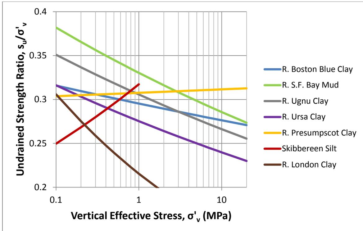
**Fig. 1:** Variation in undrained strength ratio with stress level for seven normally consolidated mudrocks. The actual data points used to produce the regression lines are omitted from the figure for clarity.
