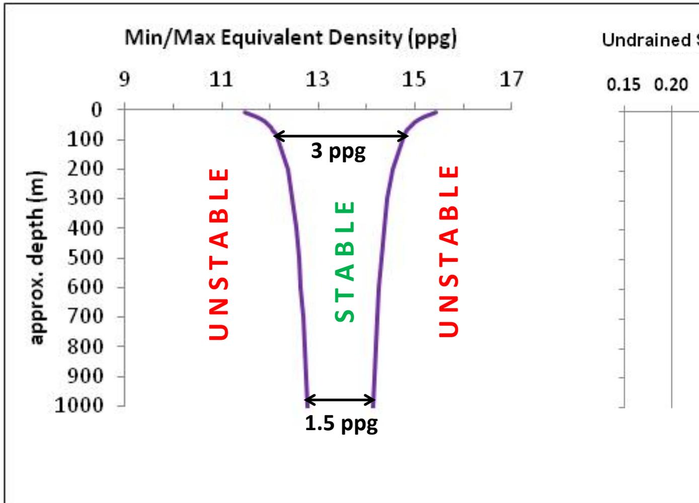
**Fig. 2:** The effect of the decrease in the undrained strength ratio of Gulf of Mexico Ursa Clay on the size of the safe drilling window for this mudrock. The minimum and maximum well pressures (in pounds per gallon) are calculated assuming a vertical well, hydrostatic water pressures and an impermeable borehole wall.
