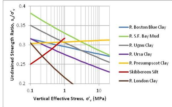
**Fig. 1:** Variation in undrained strength ratio with stress level for seven normally consolidated mudrocks. The actual data points used to produce the regression lines are omitted from the figure for clarity.
