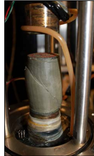
Fig. 1: Failure plane for a resedimented BBC soil specimen tested in a triaxial device.
