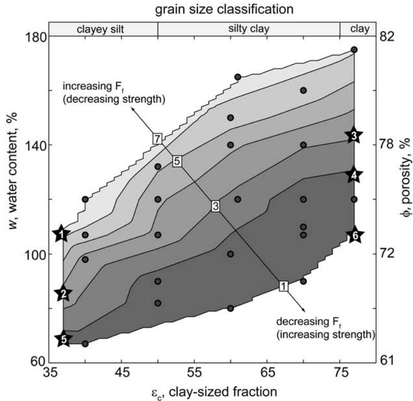
**Fig. 1:** Flow factor contour plot.
