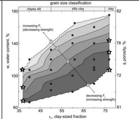
**Fig. 1:** Flow factor contours are overlain on a cross plot of clay fraction ( $\epsilon_c$ ) versus water content ( $w$ ) (and porosity,  $\phi$ ). Flow factor is determined by the ratio of gravitational shear stress to yield strength (determined by viscometer). Figure 2 shows results of experiments 1 (high  $F_f$ ), 3 (med.  $F_f$ ), and 4 (low  $F_f$ ).
