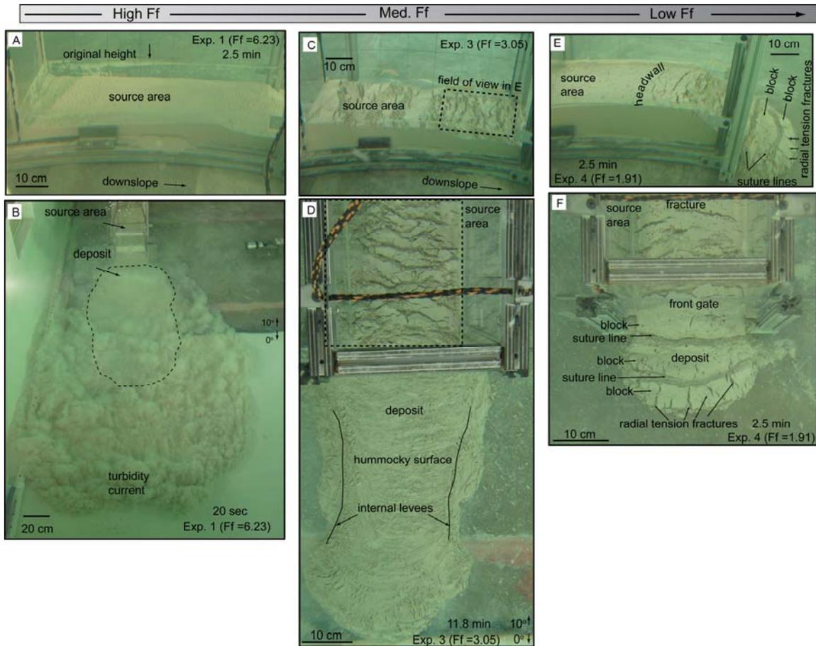
**Fig. 2:** Characteristic features of flow experiments.
