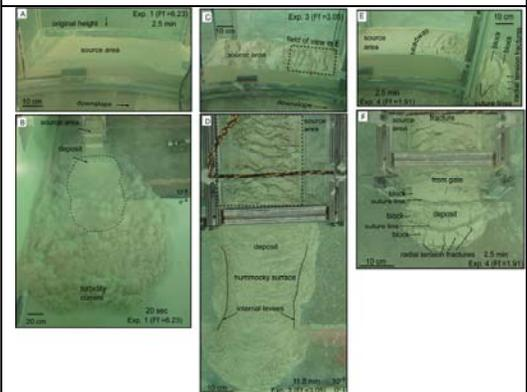
**Fig. 2:** **A, B:** High  $F_f$  mudflow produced a rapid mudflow that accelerated away from the source area and produced a prominent turbidity current. **C, D:** Medium  $F_f$  produced a long-duration (11.8 minutes) retrogressive failure. **E, F:** Low  $F_f$  produced a short-duration (2.5 minutes) blocky failure.
