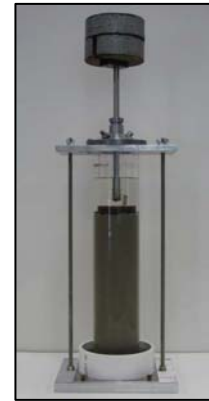
Fig. 1: Resedimentation technique whereby a slurry containing the target soil is incrementally consolidated over a certain timeframe
