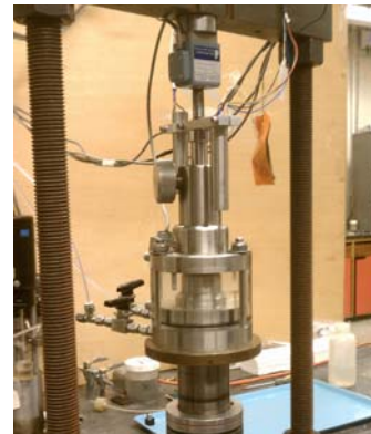
Fig. 2: Constant Rate of Strain (CRS) cell in which the compressibility characteristics of mudrocks at varying salt contents will be determined at differing stresses
