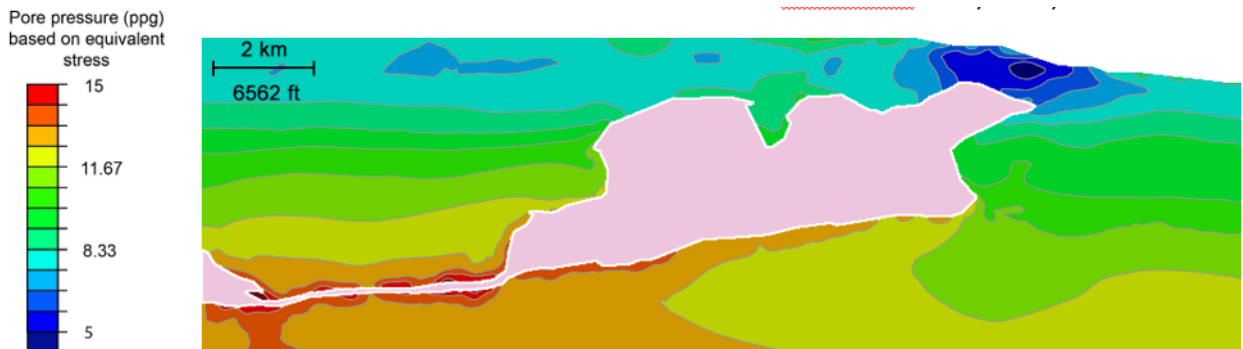
Fig. 4: UT GeoFluids has developed a workflow to couple geomechanical modeling with seismic velocity to predict pore pressure and the complete stress field in complex geologic settings (e.g., around salt bodies).
