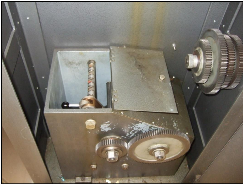
Figure 5-2: The strain rate on the Wykeham Farrance load frames is set by adjusting the cog combination.
