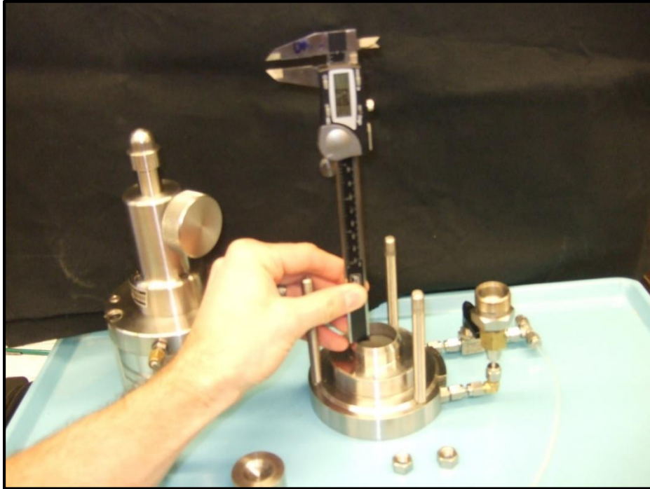
Figure 5-11: After replacing the acrylic spacer with the top porous stone (SSD), the depth of the porous stone within the confinement ring is measured using calipers.
