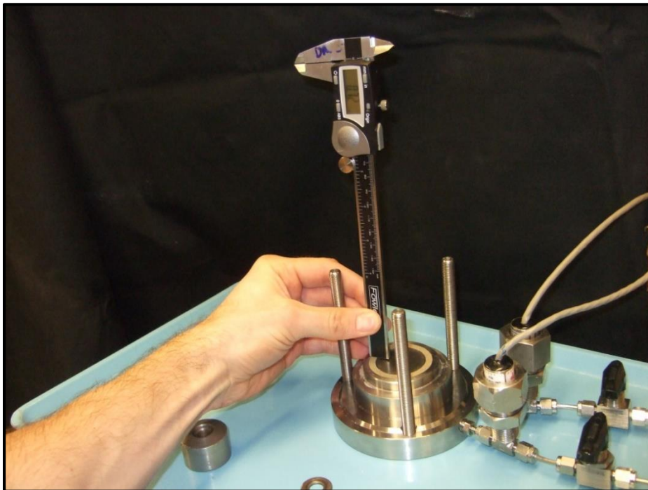
Figure 5-26: The depth of the top cap within the confinement ring is measured using calipers.
