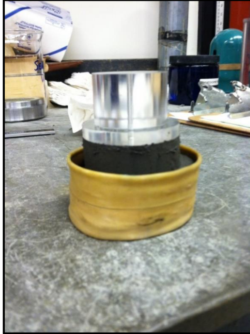
Figure 3-23: A smaller specimen is cored out of the larger specimen sheared in the DSS device using piano wire and acrylic cylinders as guides.
