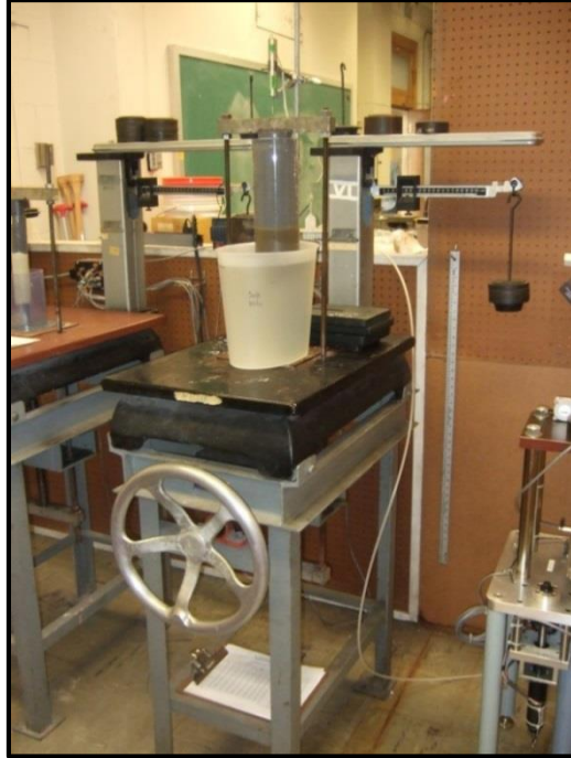
Figure 3-15: A consolidometer with a 100:1 lever arm is used to compress specimens from about 0.1 to 1.5 MPa. The lever arm magnifies the load provided by the weights.
