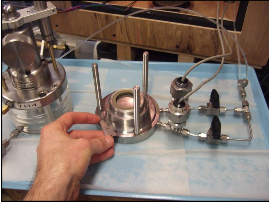
Figure 5-31: The use of a blade can help remove the confinement ring, specimen, and top cap from the base.
