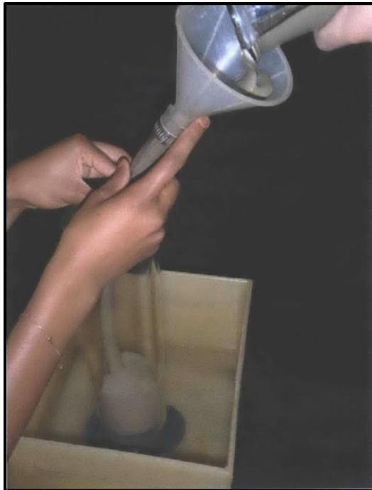
Figure 3-12: Soil slurry is carefully tremmied into acrylic sedimentation column prior to loading (Adams, 2014).
