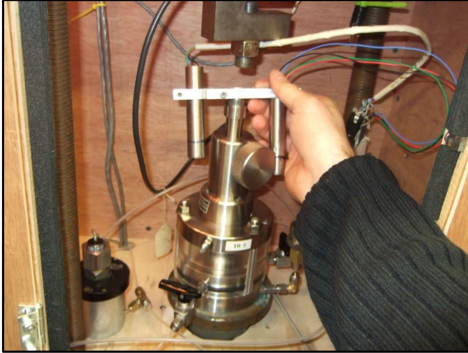
Figure 5-13: The LVDT hanger (attached to the LVDTs) is fastened onto the piston.
