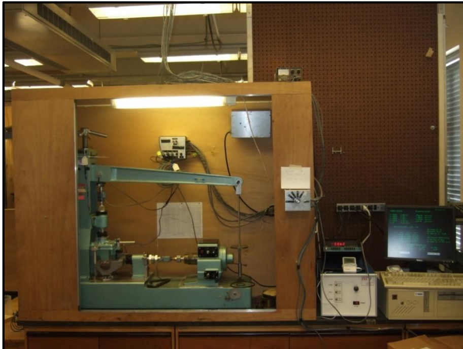
Figure 3-20: A DSS device is used to shear the samples in uniform horizontal simple shear. This is thought to create more fabric anisotropy than vertical compression alone.
