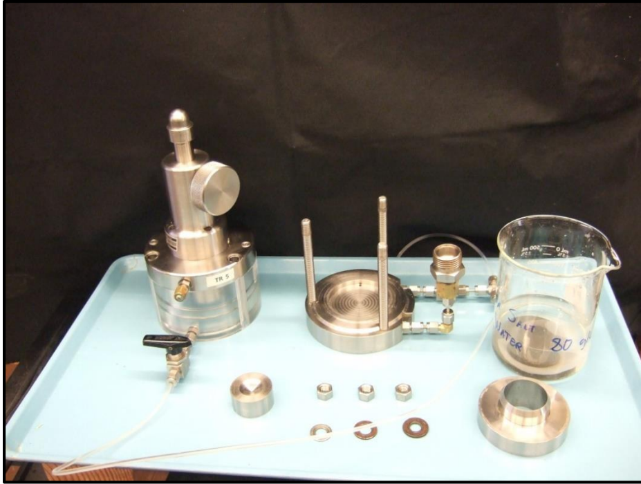
Figure 5-1: The vertically-draining CRS apparatus is disassembled and prepared prior to specimen trimming.
