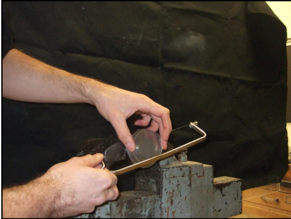
Figure 5-9: The bottom of the specimen is trimmed by placing the confinement ring in a bench-mounted vice. The plastic disc aids in removing the trimmed soil.
