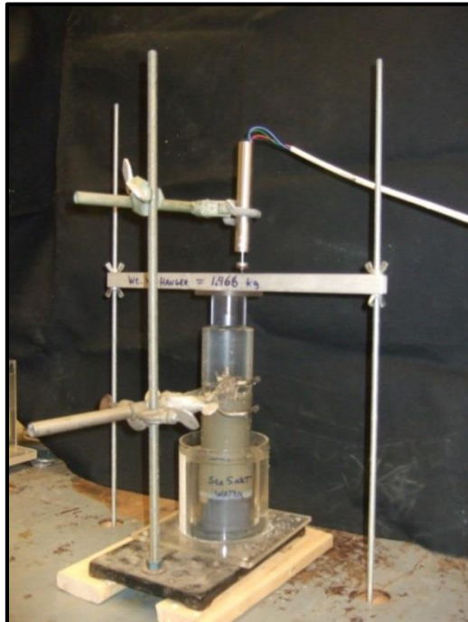
Figure 3-14: An LVDT is connected to the consolidometer to measure vertical settlement.
