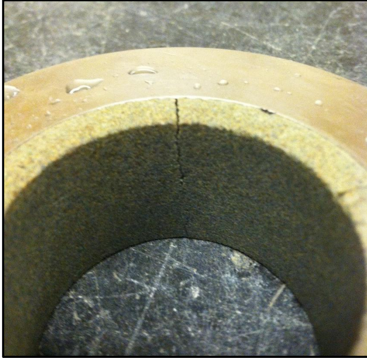
Figure 4-4: The epoxied porous stone cracked during trial loading.
