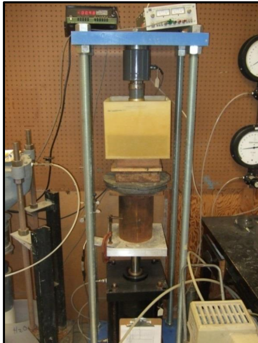
Figure 3-16: An air-pressure controlled load frame is used to compress specimens up to about 10 MPa. An air-pressure actuator at the base applies a load and a load cell at the top measures it.
