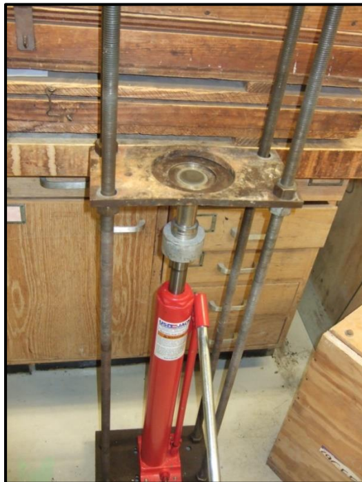
Figure 5-32: A hydraulic jack can be used to extrude the specimen and top cap from the confinement ring.
