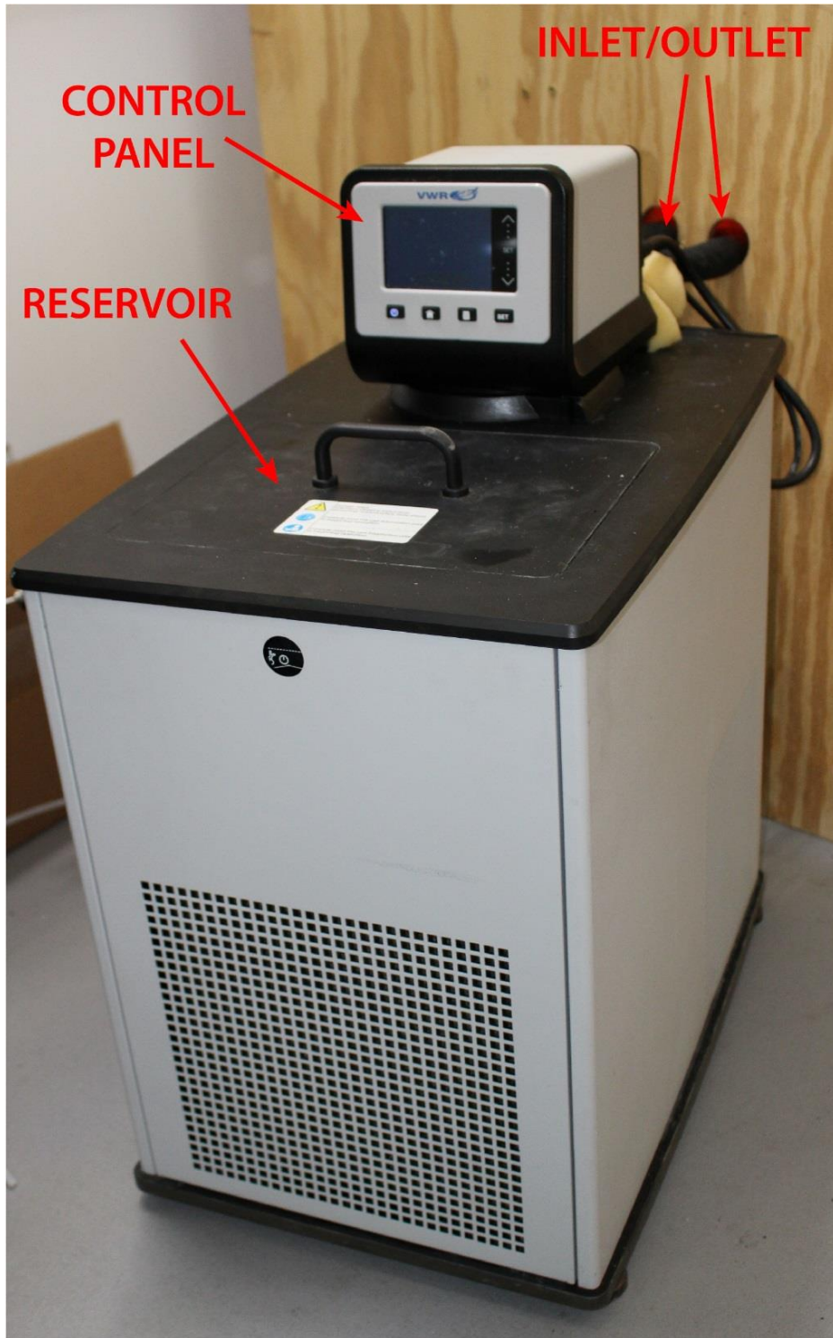
Figure A.7: Picture of chiller.
