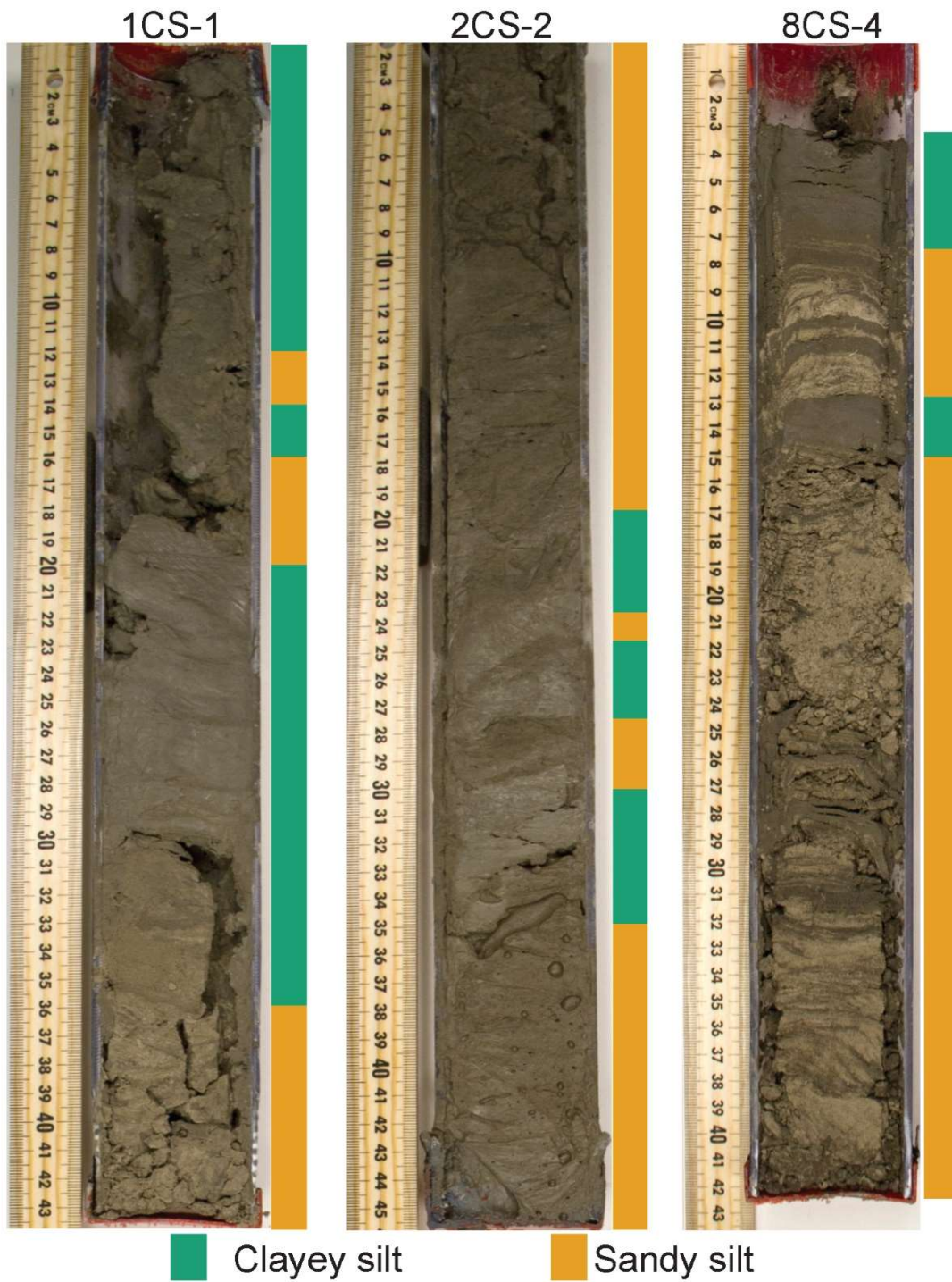
Figure 10. Photographs of split, non-pressure cores from H002. 1CS-1 is from unit 1, immediately above the hydrate reservoir (Figure 4). 2CS-2 spans the boundary of unit 1 and unit A. 8CS-4 is from unit A.
