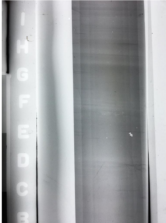
Figure 23. X-ray image of intact Boston Blue Clay. Letters are spaced 1-inch apart and correspond to markings along the length of the steel tube. The sample quality of this section is superb, as the layers are completely horizontal and there are no rocks or cracks present. More damaged intact samples will show bent layers or large voids due to sampling. Sampled section for triaxial testing is about from markings D to G.
