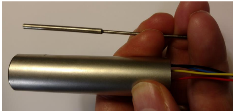
Figure 46. LVDT. The core sliding in the tube produces a DC voltage change proportional to displacement in the linear range. Photo from Dr. Germaine's CEE 244 Course notes.
