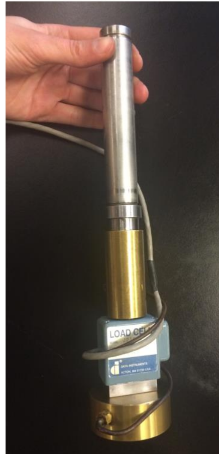
Figure 47. Cross section of the triaxial cell (left) shows the internal components. The piston setup can be seen on the right, where the load cell is nearly in direct contact with the specimen.
