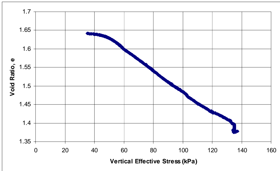
Figure A.23: Void Ratio Versus Vertical Effective Stress – Triaxial Test # 801
