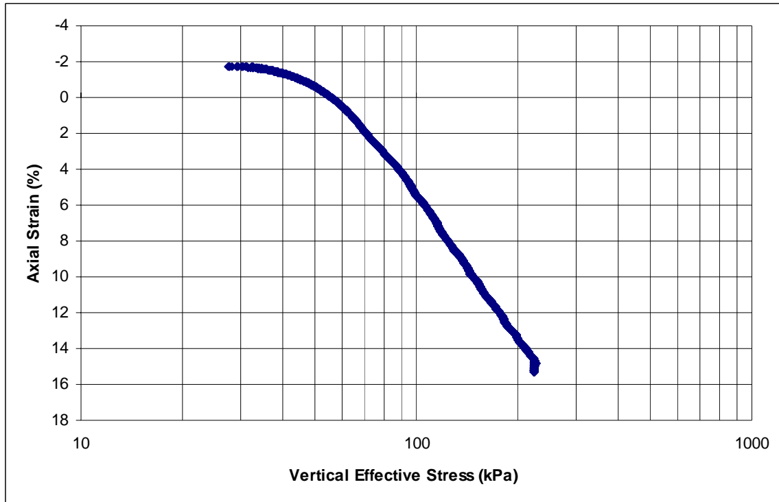
Figure A.3: Axial Strain Versus Vertical Effective Stress – Triaxial Test #804
