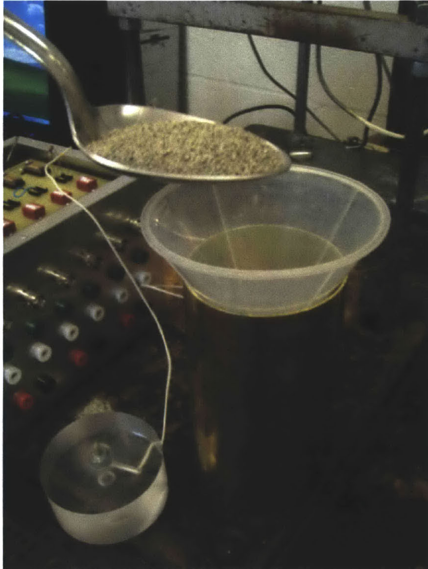
Figure 3-1: The specimen of Ticino sand is prepared using a funnel and the rodding method, which involves using a long slender rod to puncture the sand and ensure uniform distribution. This is performed in three stages.
