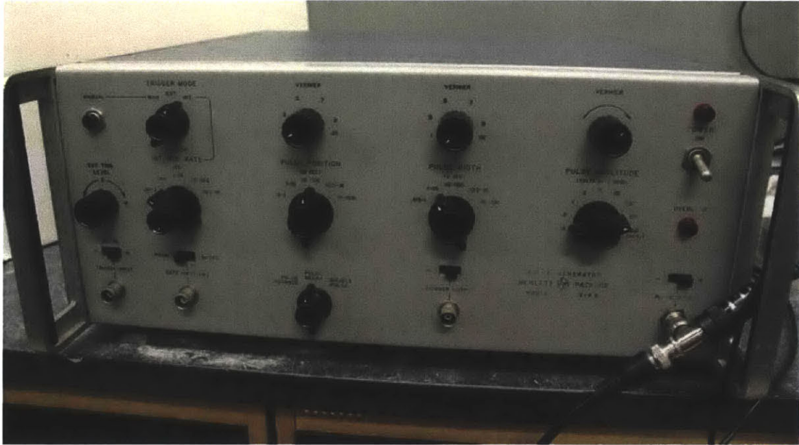
Figure 4-10: This square pulse generator sends a high voltage high frequency pulse to the P-wave transducer to propagate a signal
