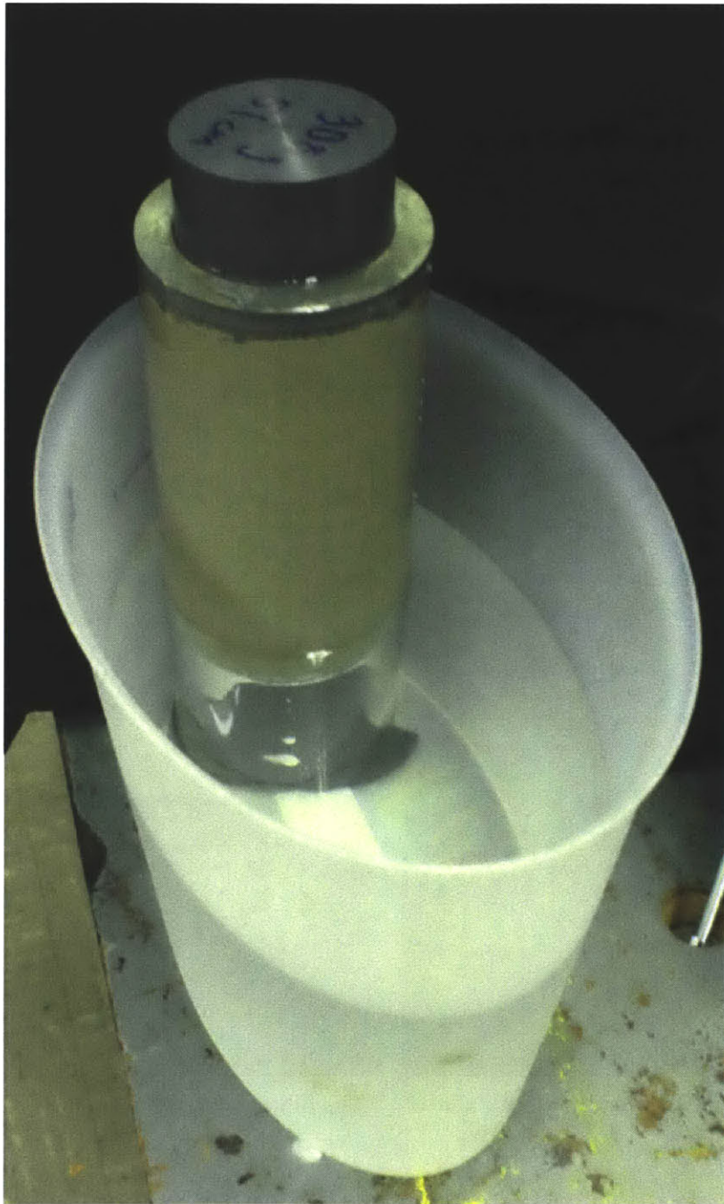
Figure 3-10: Post-funneling, a porous stone and incremental spacers are added on top of the slurry to begin the resedimentation process. It sits in a salt water bath (at the same salt concentration as the slurry was made) with double-drainage access.
