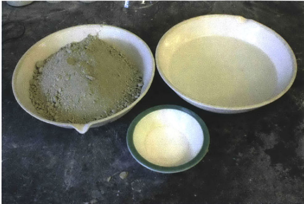
Figure 3-6: Three components used to mix the slurry: sea salt (16g/L), ground BBC (1000g), distilled water (1L).
