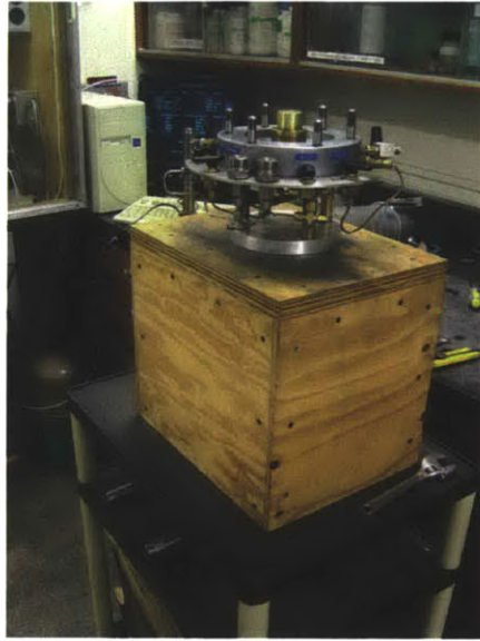
Figure 4.18: The base of the high pressure triaxial apparatus resting on the mobile cart.
