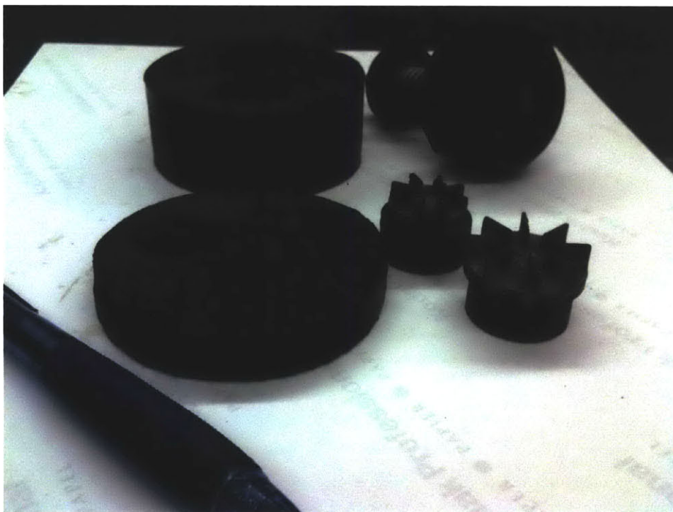
Figure 4.7: The Torvane testing device; using a small and medium vane on SFBM to estimate shear strength.
