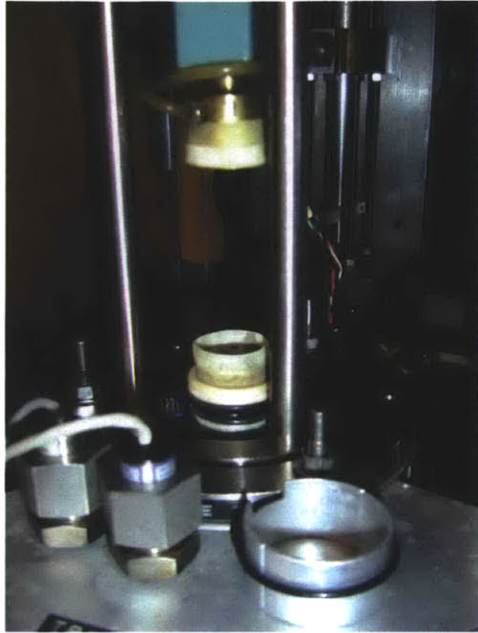
Figure 4.8: The pedestal and top cap with the rubber sleeves and rolled condom in place.
