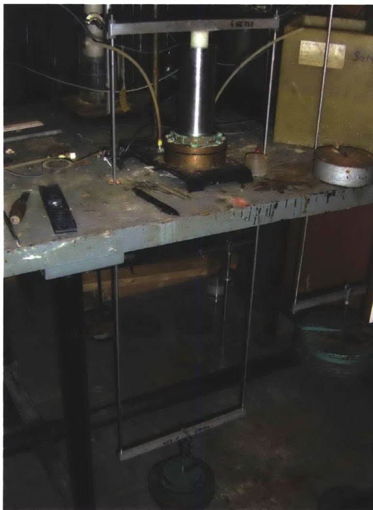
Figure 3.5: Incremental loading with free weights at a modified oedometer base - consolidometer.
