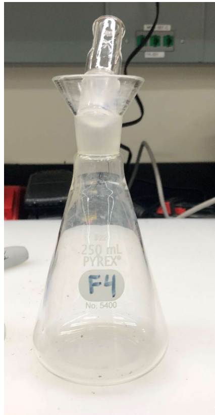
Figure 4-5: Specific gravity flask
