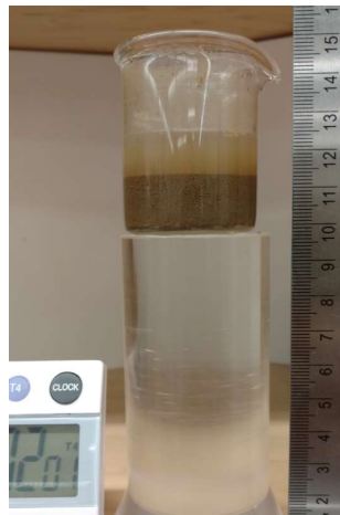
Figure 3-6: Primary processed material fast settling rate
