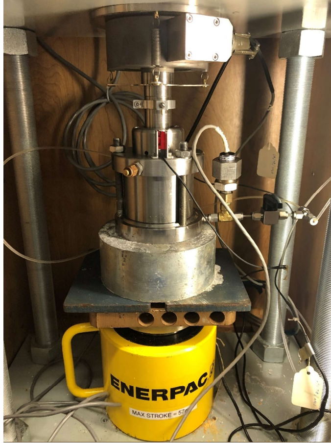
Figure 4-15: High stress CRS cell
