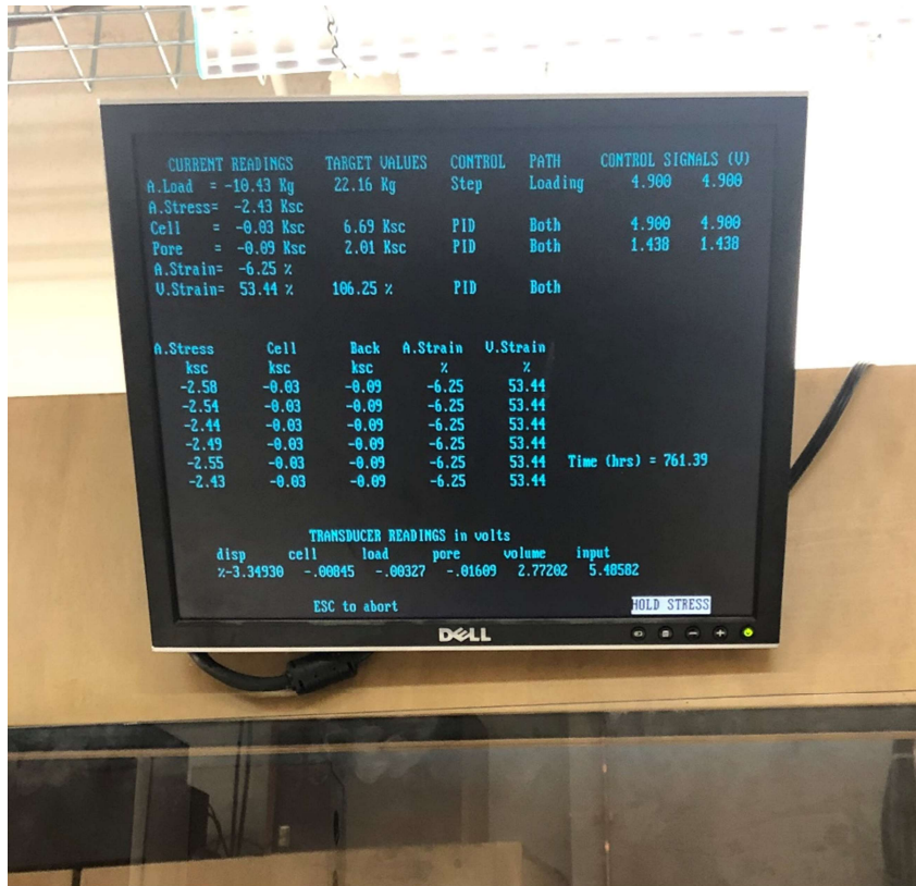
Figure 4-8: Computer control monitor and user interface
