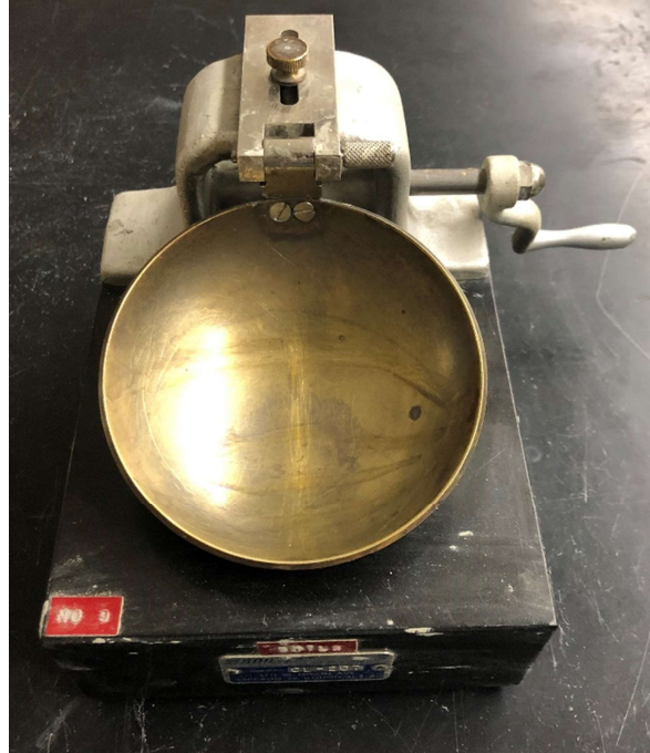
Figure 4-1: Casagrande cup for Liquid Limit Test
