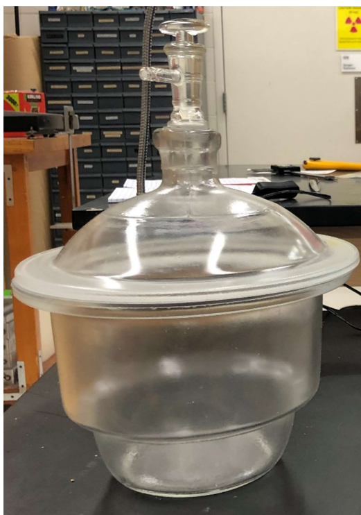
Figure 3-12: Vacuum desiccator used for saturating intact samples
