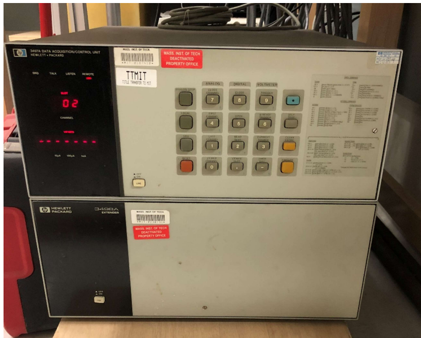
Figure 4-7: Tufts central data acquisition system
