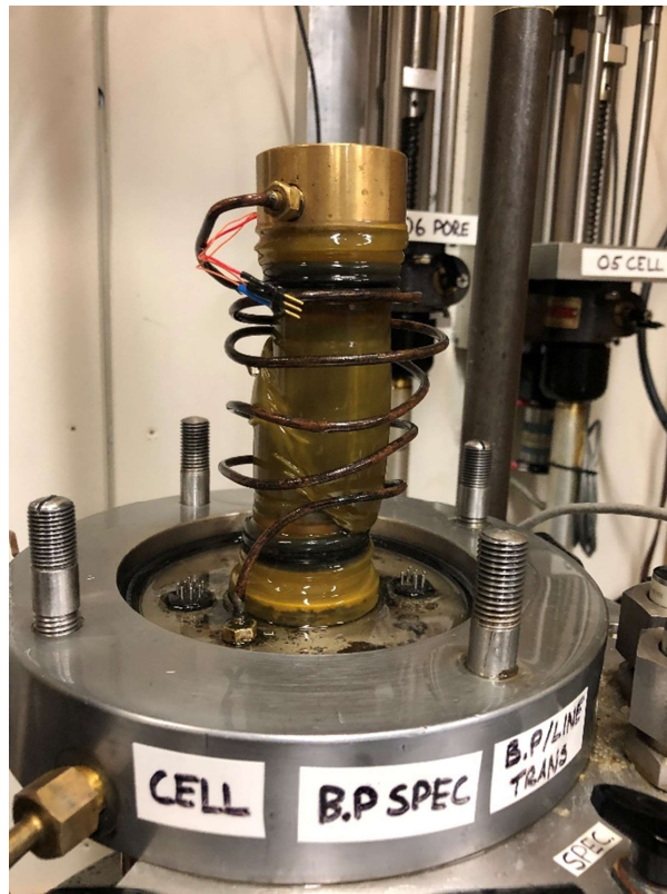
Figure 5-38: Failure plane in medium stress specimen
