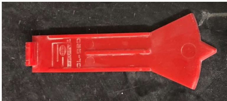
Figure 4-2: Liquid limit grooving tool
