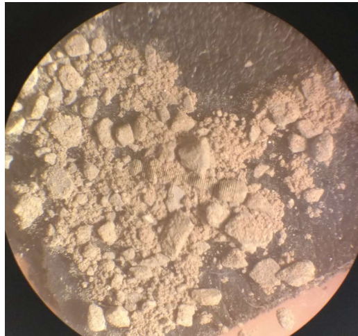
Figure 3-4: Primary processed material with intact clay aggregates
