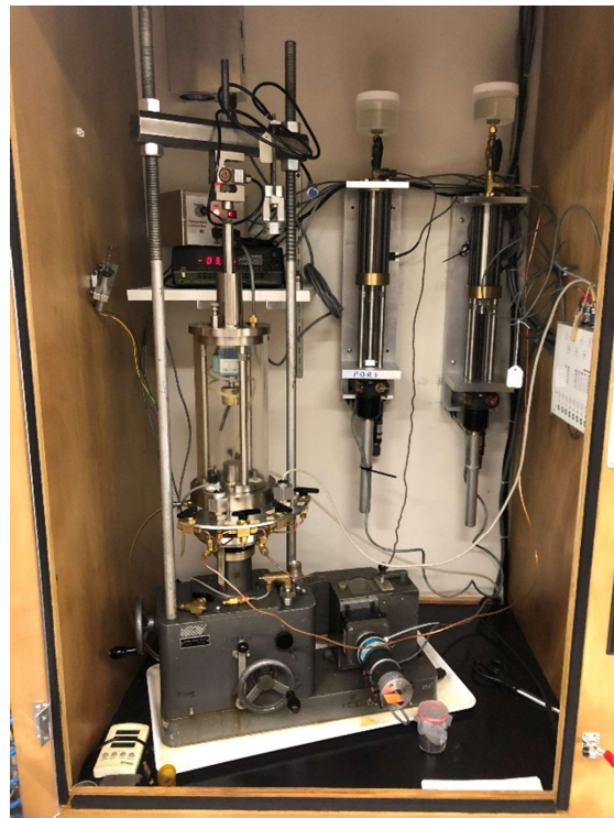
Figure 4-17: Low stress triaxial cell
