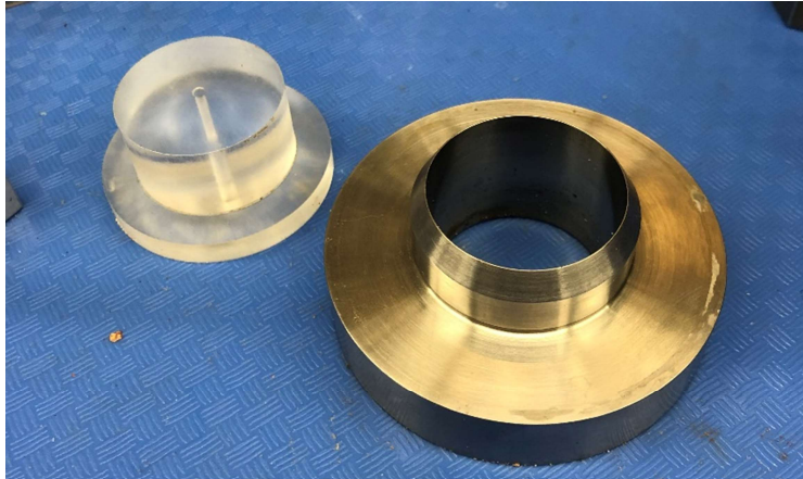
Figure 4-12: CRS confining ring and recess tool
