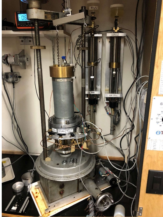
Figure 4-18: Medium stress triaxial cell
