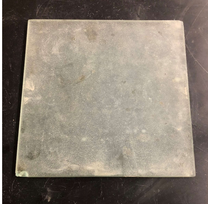
Figure 4-4: Plastic limit grooved glass plate
