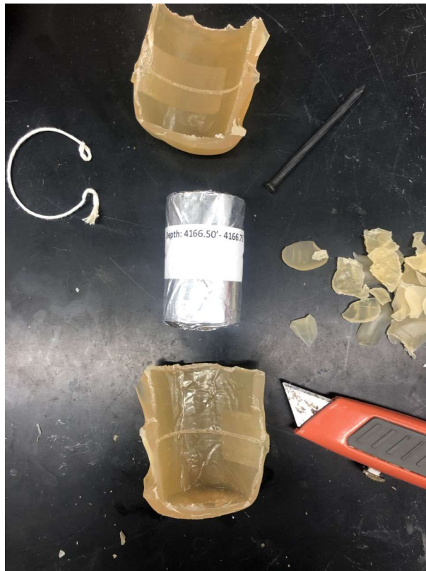
Figure 5-22: Intact CRS specimens
