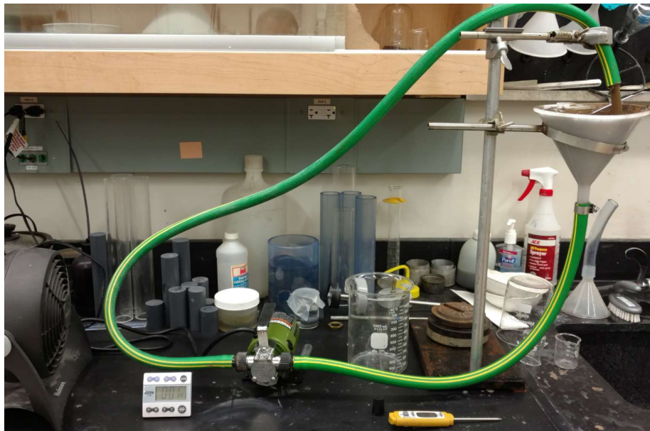
Figure 3-8: Shear pump circulation apparatus
