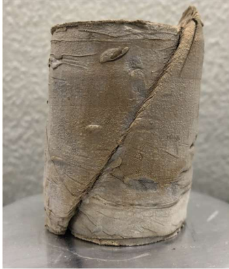
Figure 5-37: Failure plane in low stress specimen
