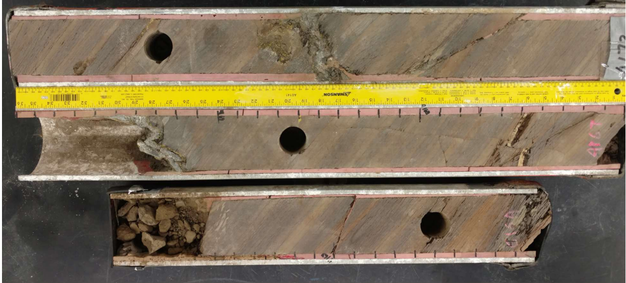
Figure 3-1: Non-preserved core samples as received in the Tufts Laboratory from Chevron
