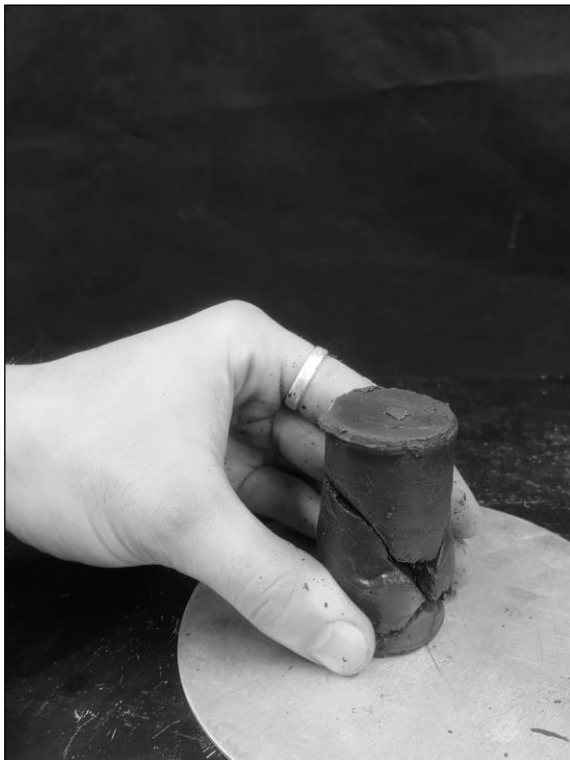
Figure 6-12 – Two images showing specimen from triaxial test TX1476. The specimen was run first in triaxial extension, and then in triaxial compression.
