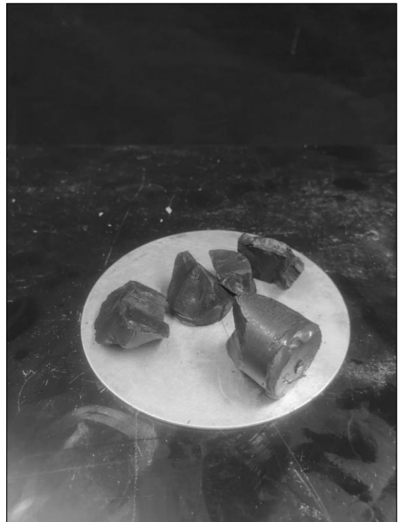
Figure 6-12 – Two images showing specimen from triaxial test TX1476. The specimen was run first in triaxial extension, and then in triaxial compression.
