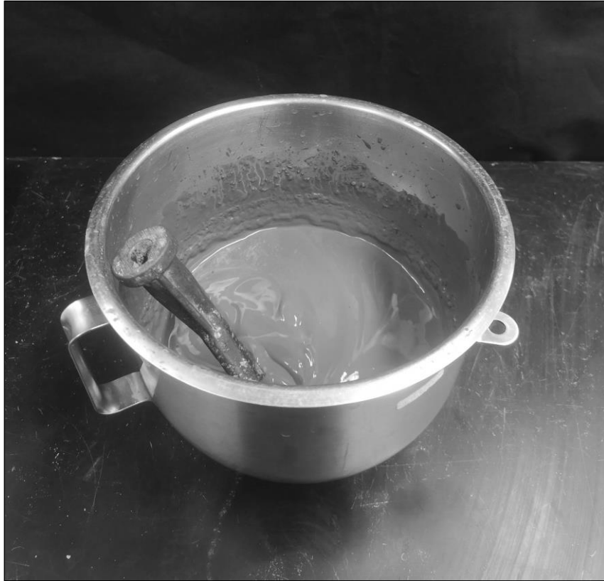
Figure 3-6 - Image showing GoM-EI clay powder after mechanical mixing with salt and water.
