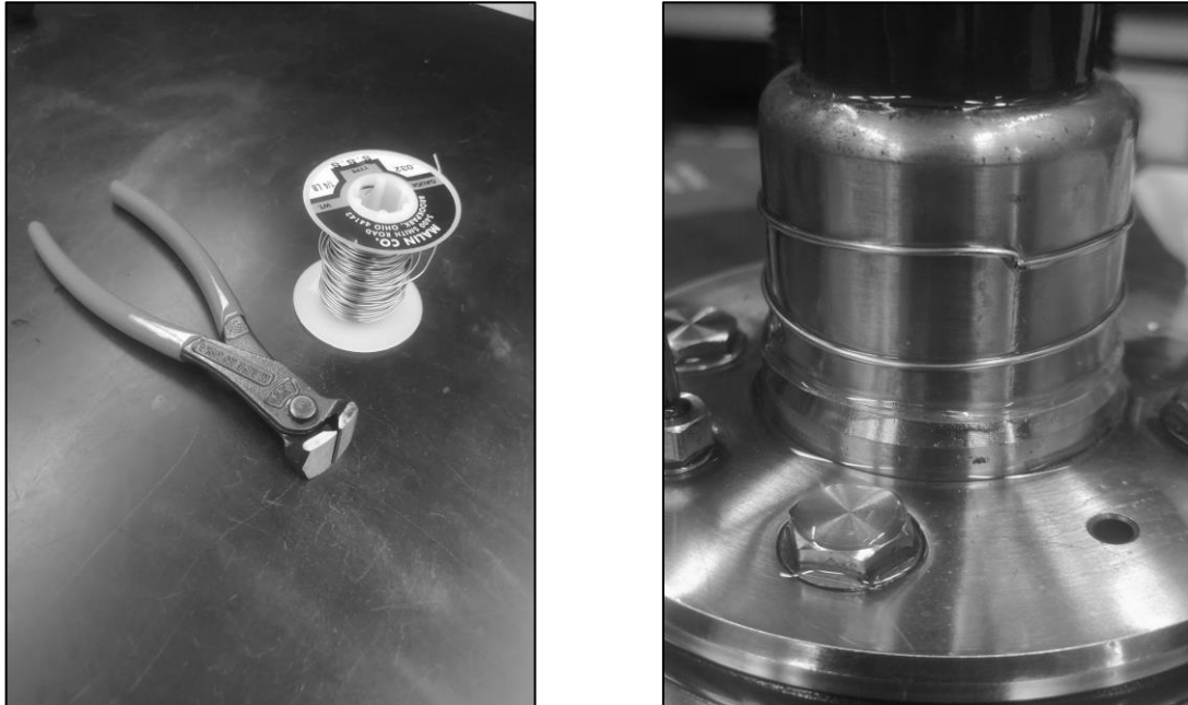
Figure 5-1 - Image showing steel tying wire (Left) and the tying wire used to create a seal between the PVC membrane and base pedestal (Right)
