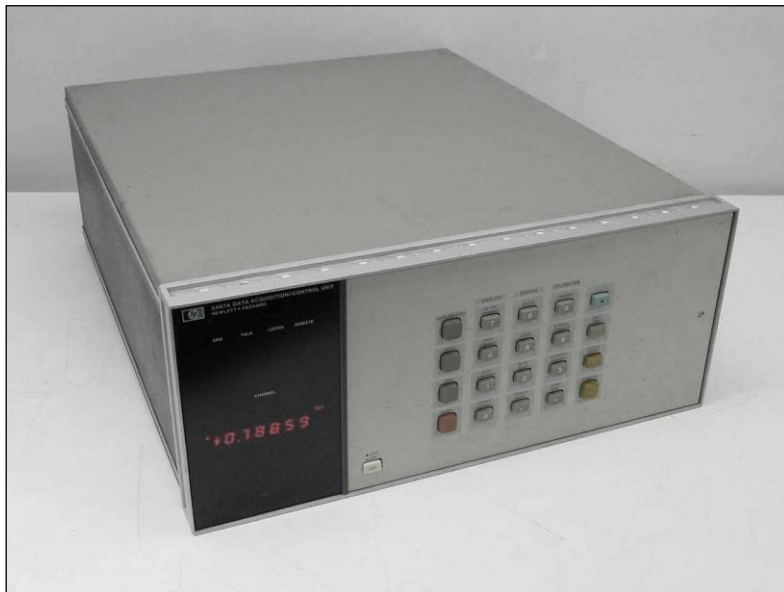
Figure 4-11 - HP 3497A data acquisition control unit, used to capture readings from the high pressure cell
