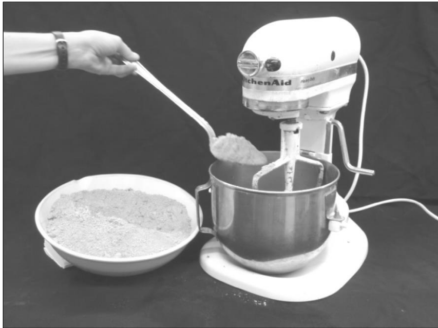
Figure 3-5 - Image showing mixing of a clay powder, taken from (Casey 2014).
