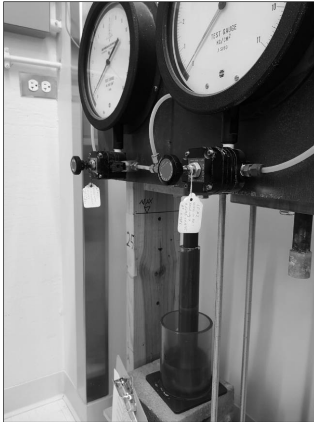
Figure 3-9 - Image showing a pneumatic actuator, which permits consolidation from between 0.25 - 5 MPa.
