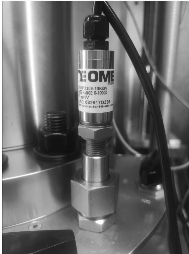
Figure 4-5 - Image of pore pressure transducer located on the base of the high pressure triaxial cell.
