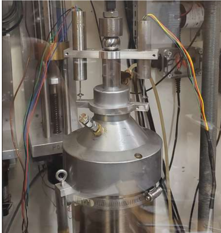
Figure 5-4 Two LVDTs used to measure specimen axial displacements on the medium pressure triaxial system Station 6
