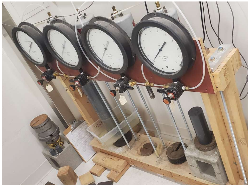
Figure 4-3 Pneumatic piston system used for maximum loads of 400 kg.
