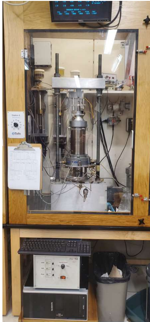
Figure 5-1 Medium pressure triaxial system enclosed in temperature control box at Station 6.
