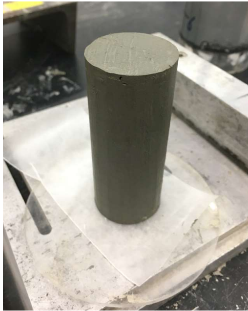
Figure 4-5 Trimmed RBBC sample ready for triaxial testing.
