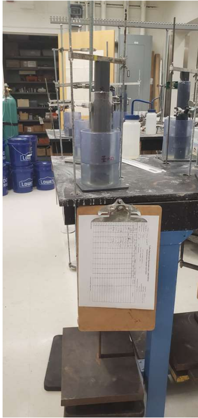
Figure 4-2 Hanger system utilized for early stages of consolidation with maximum load of 40 kg.
