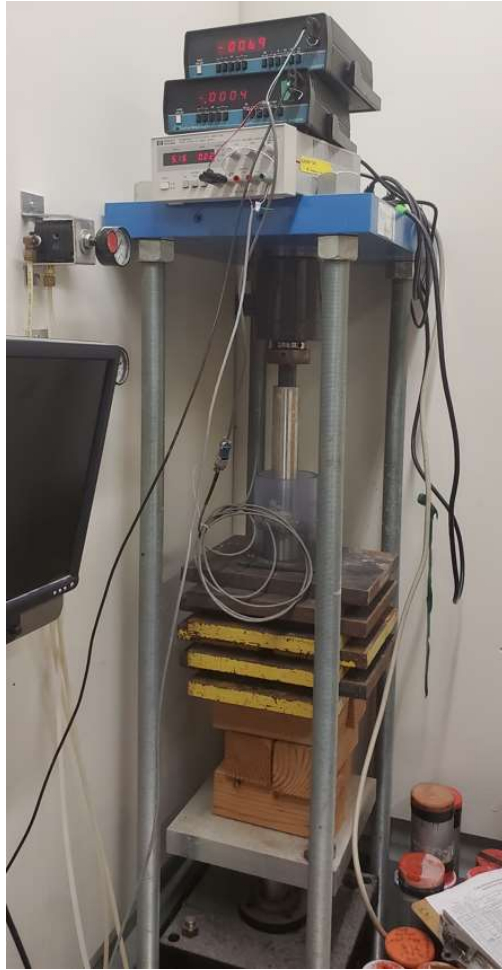
Figure 4-4 Pneumatic load frame used for consolidation stresses of over 8 MPa.
