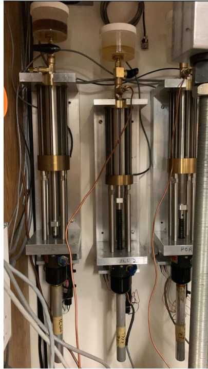
Figure 5-5 14 MPa capacity PVAs utilised at Station 6.
