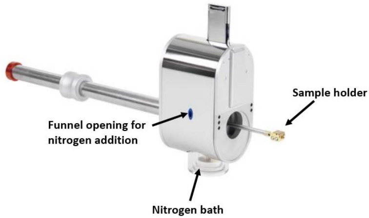
Figure 4-8: Vacuum-cryo-transfer system (VCT, #EM VCT100, Leica Microsystems, Vienna).
