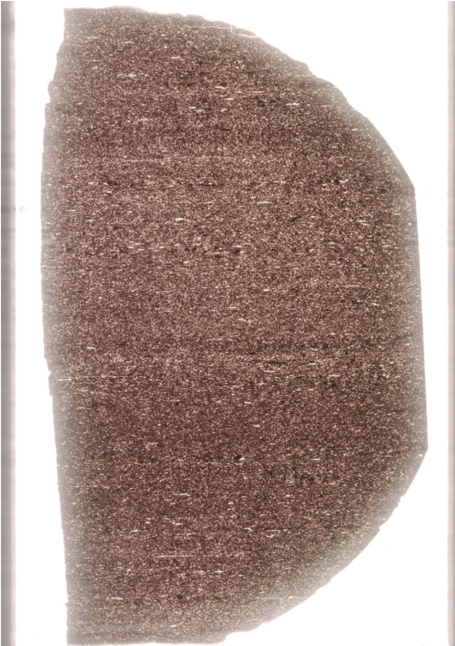
Figure 4.3 High-resolution scanned image of BAR6H1_ET thin section. This thin-section was prepared from an end trim of the 6H1 core plug. Re-worked Ca-phosphate-rich grains (maroon colored) and shell fragments (white) tend to concentrate in thin intervals.
