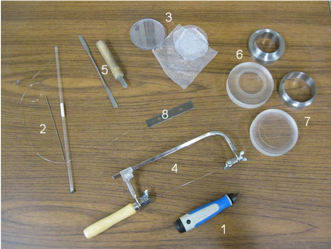
Figure E1: Tools used in CRS sample preparation
