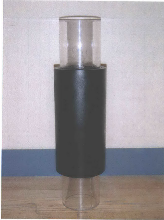
Figure 3-10: Steel reinforced sedimentation tube (without protective rubber membranes)
