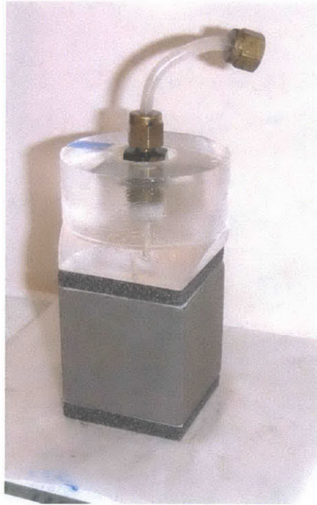
Figure A2-15: Specimen assembled with porous stones, filter screens and top end adapter
