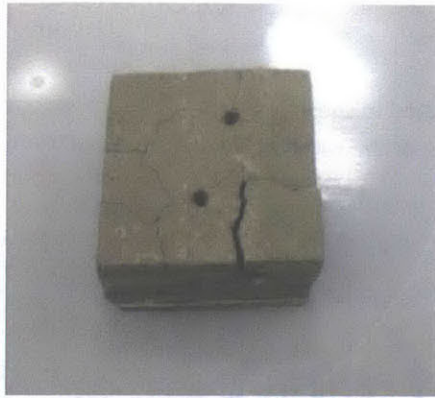
Figure A3-19: CRS specimen cracked during 4-probe pin insertion
