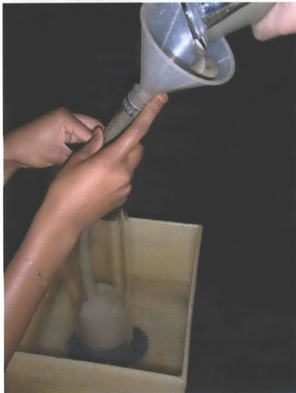
Figure 3-7: Resedimentation: Pouring the sediment slurry into 3" ID settling columns using a funnel method
