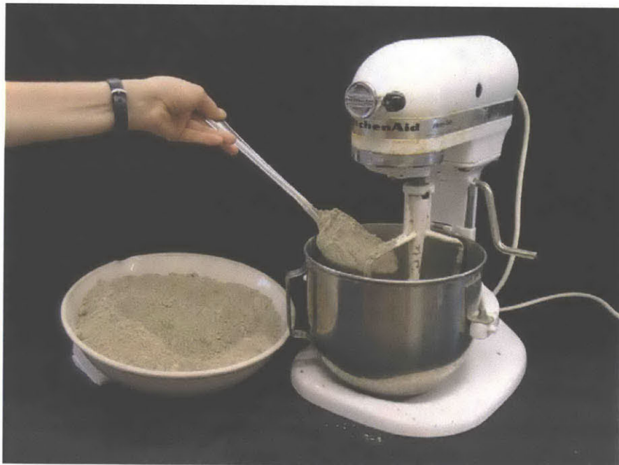
Figure 3-5: Resedimentation: Mixing dry soil powder with salt water in an electric mixer
