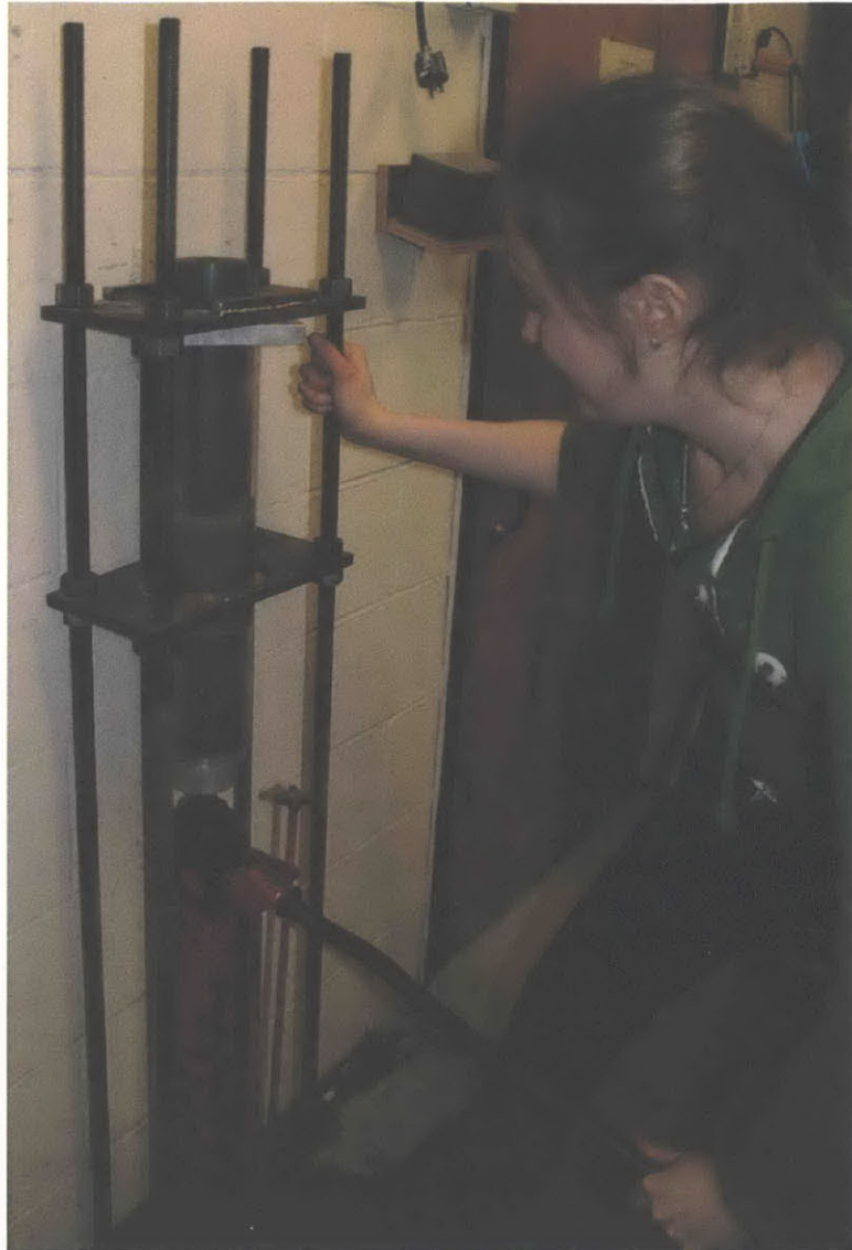
Figure A2-12: Extruding a resedimented specimen using the manual hydraulic jack
