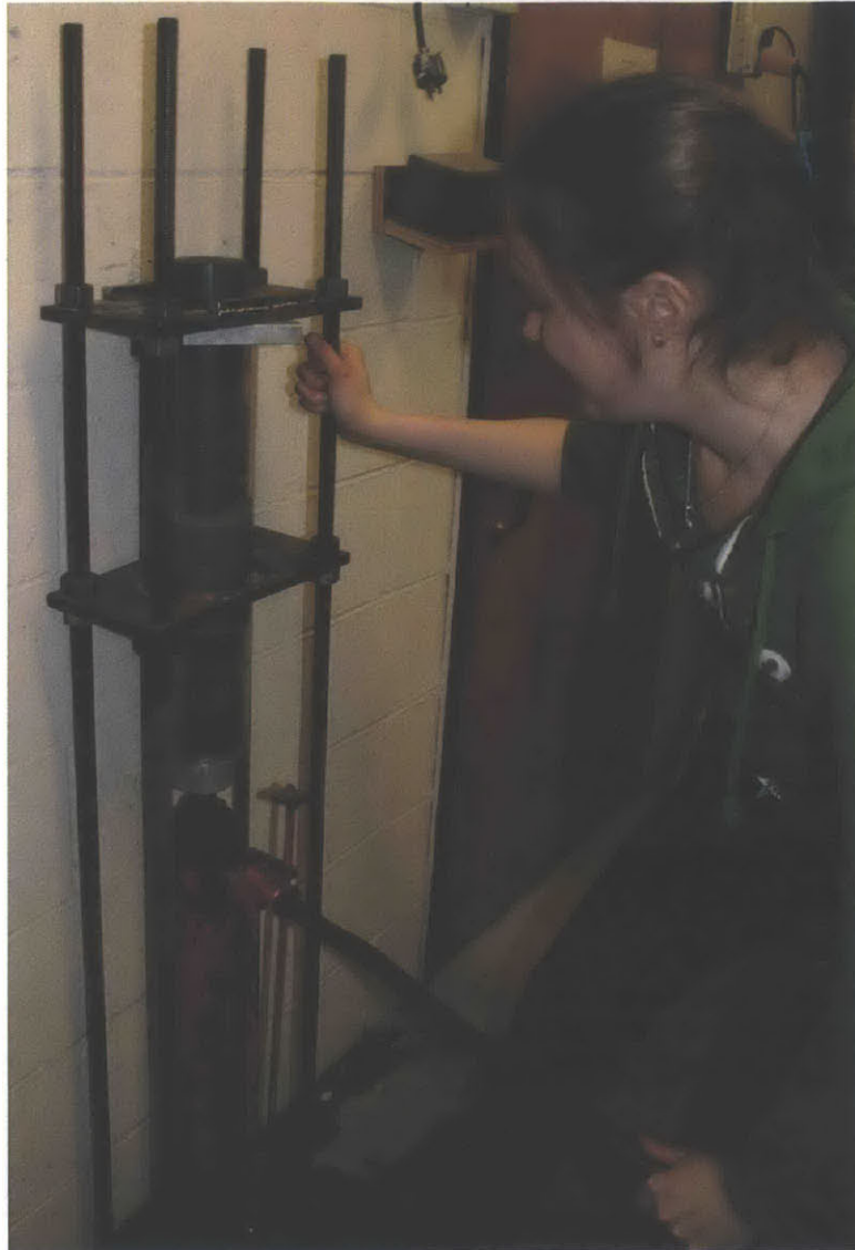
Figure 4-2: Extruding a resedimented specimen using the manual hydraulic jack
