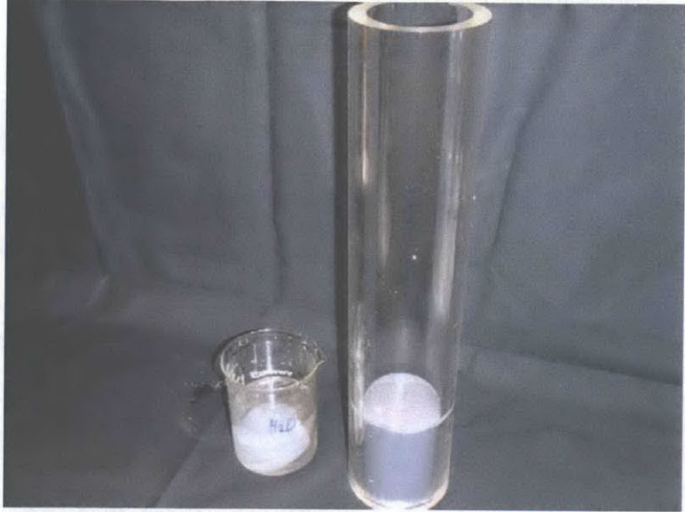
Figure 3-8: Resedimentation: Configuration of base porous stone and filter paper in sedimentation column
