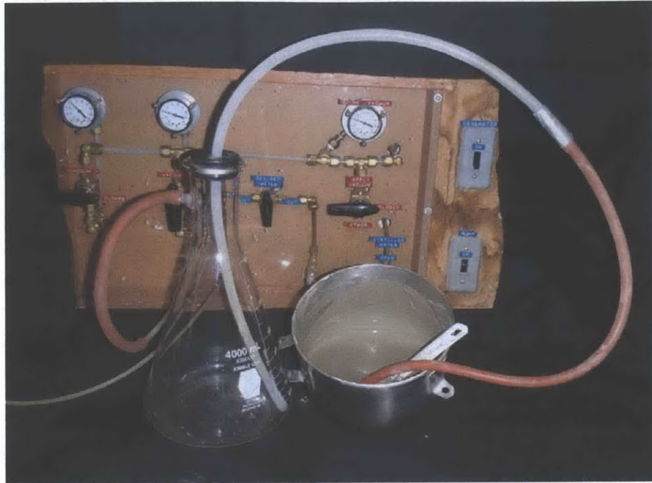
Figure 3-6: Resedimentation: Transferring the sediment slurry to a vacuum cylinder for de-airing
