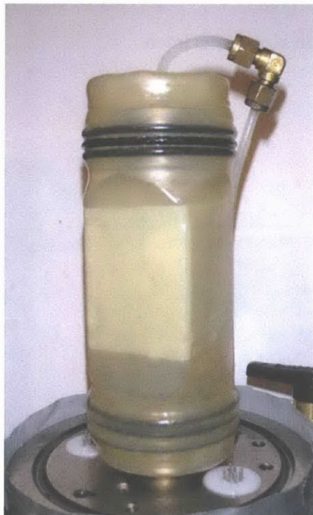
Figure A2-16: Specimen with double rubber membrane and O ring seals
