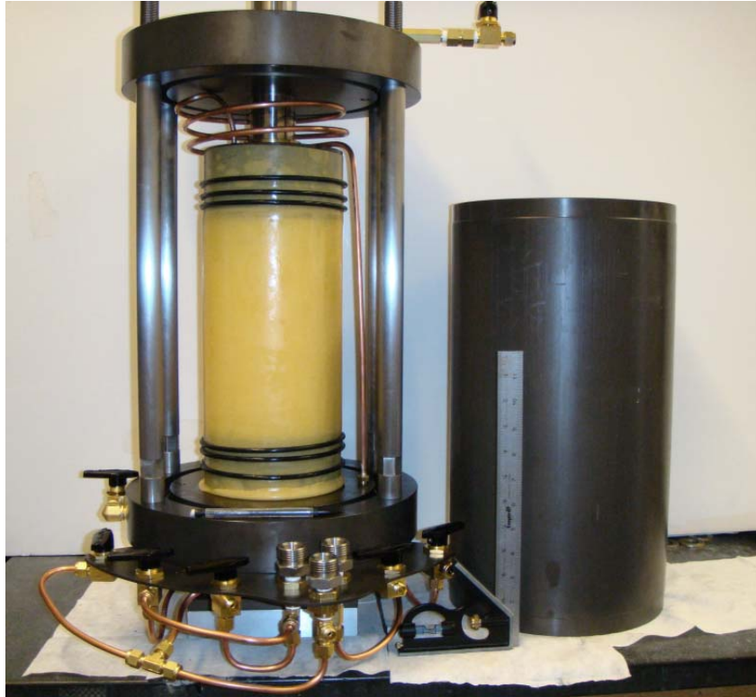
Figure 4-15: Photograph of the large diameter TWC apparatus
