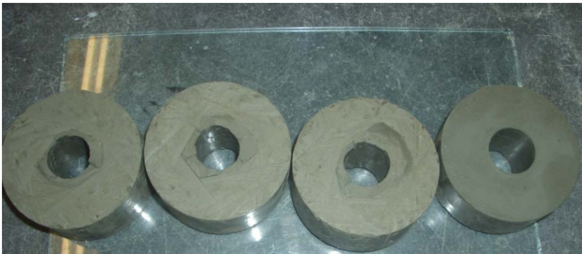
Figure 4-30: Sliced small diameter TWC specimen after test
