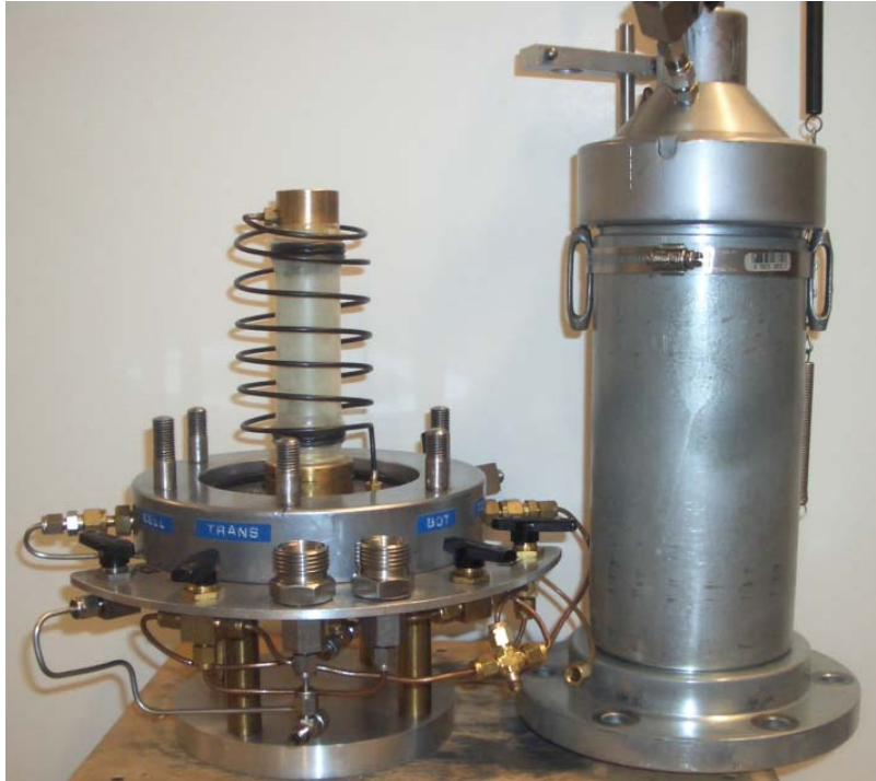
Figure 4-6: Photograph of the high pressure triaxial base and steel chamber
