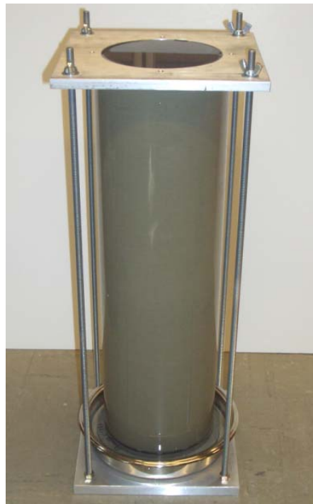
Figure 3-4: Large TWC consolidometer setup: a) schematic, b) photograph
