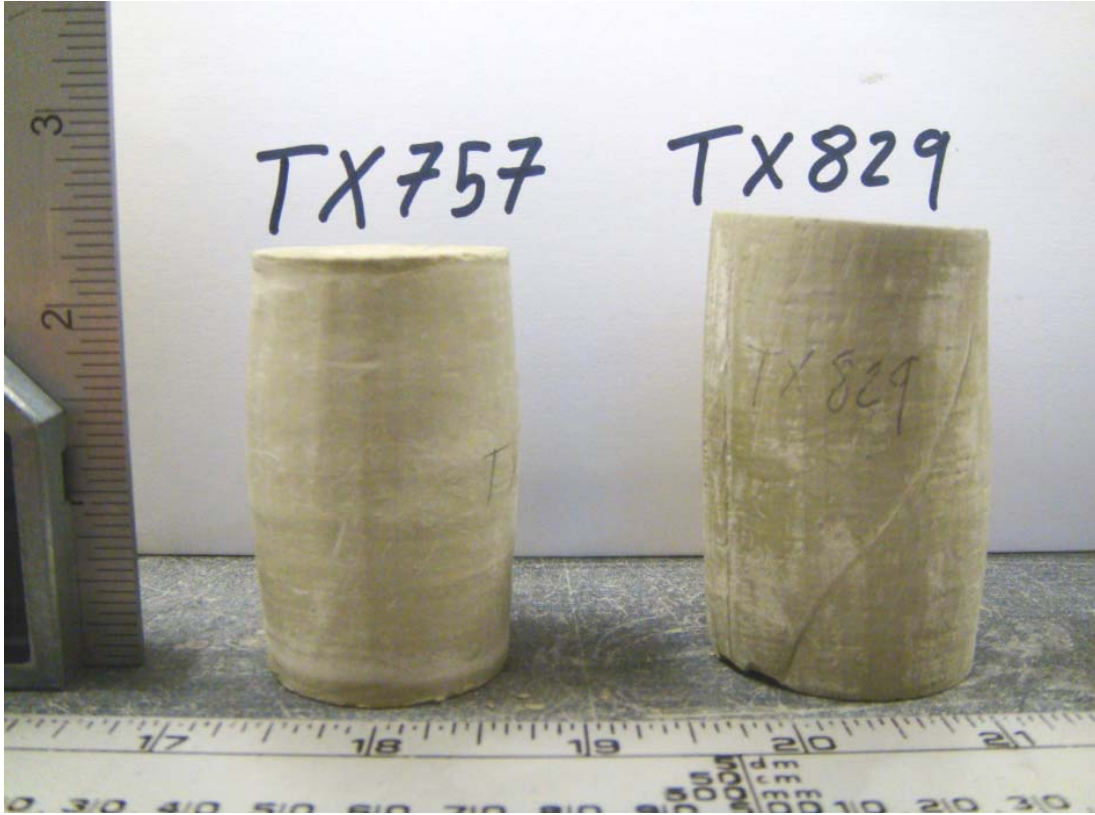
Figure 5-24: A picture of NC RBBC specimens after CK_0UC triaxial testing showing bulging mode of failure for low pressure test (left) and slip surface for high pressure test (right)
