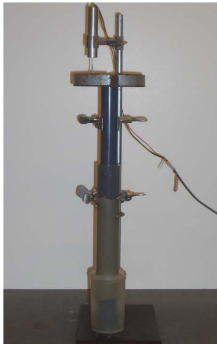
Figure 3-8: Small plexiglass triaxial consolidometer setup
