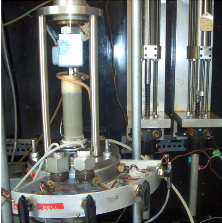
Figure 4-3: Photograph of the low pressure triaxial apparatus
