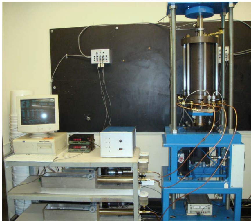
Figure 4-16: Photograph of the large diameter TWC system
