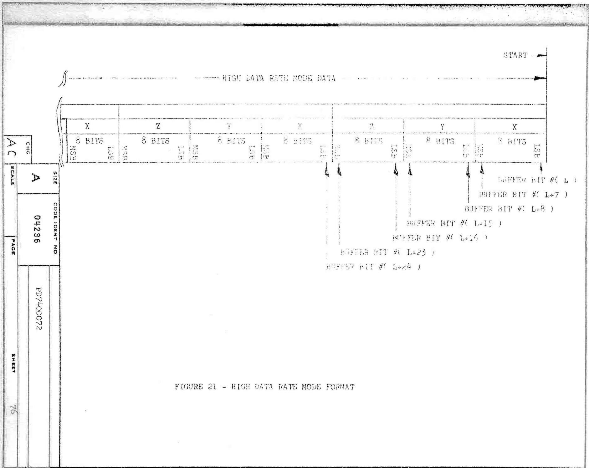
FIGURE 21 - HIGH DATA RATE MODE FORMAT
