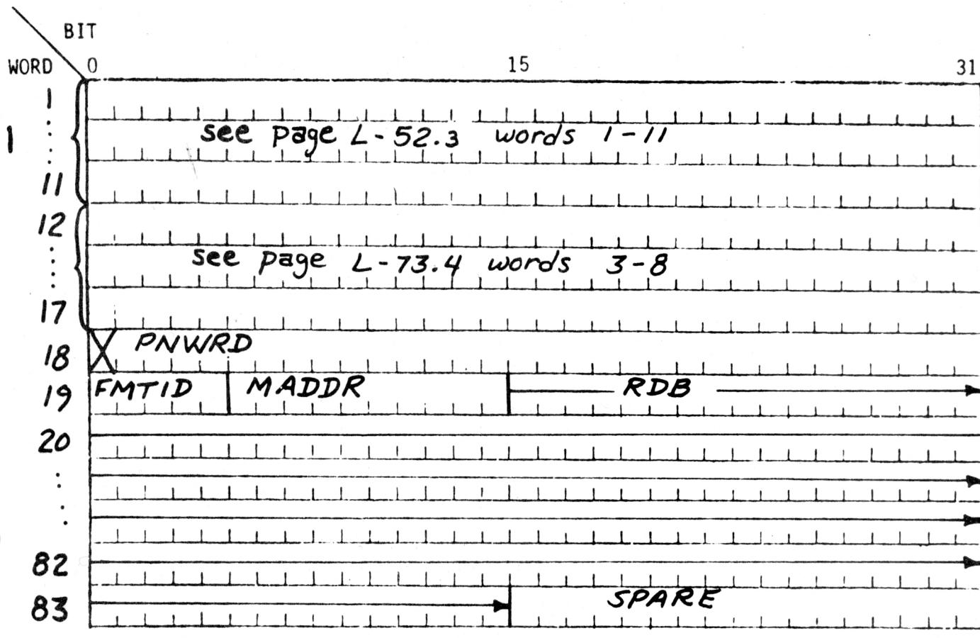
Any incomplete frames (ie. less than 83 words) will be zero filled. Lower priority seismometer data will be in the following order:
