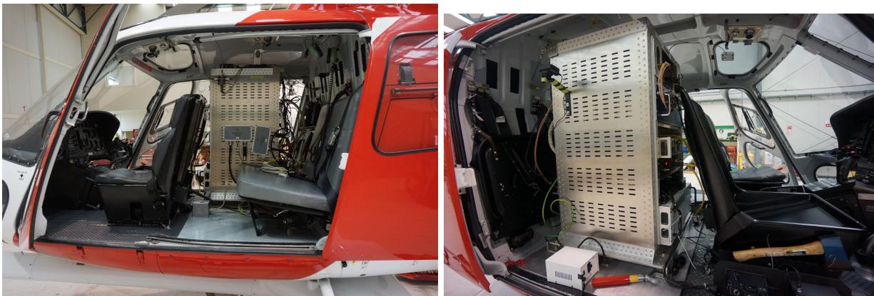
*(Top: Laser and camera mount. Bottom: The electronics rack.)*
