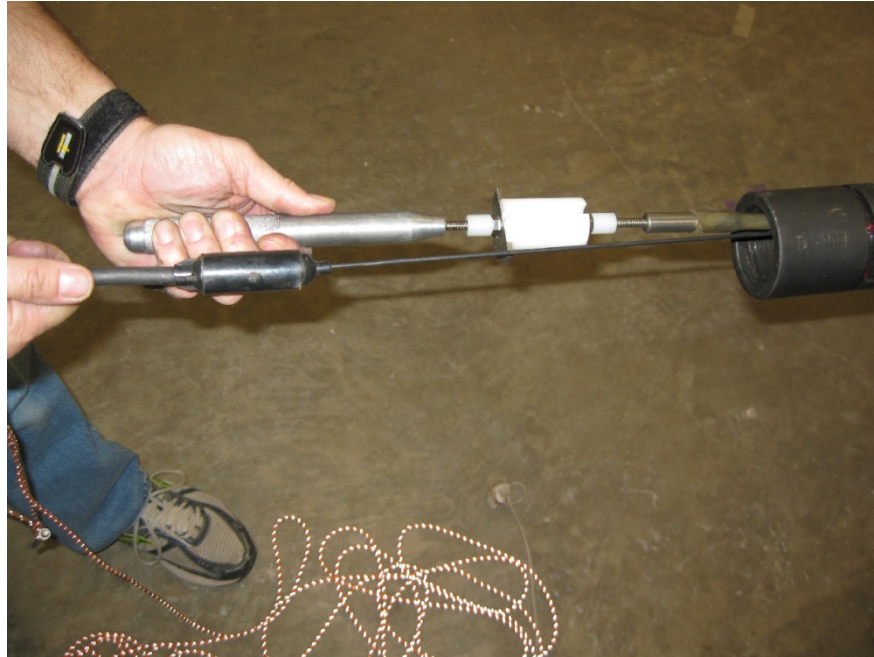
Fig. 5 Lower stopper assembly being installed using the stopper insertion tool. Note that the IE4M splice is on the downtool side of the stopper.
