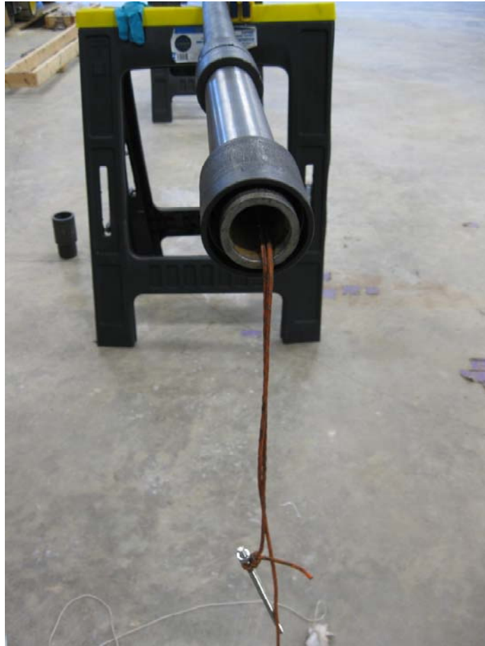
Fig 6. String remains attached to the IE4M after installing the male quick release, otherwise it is very difficult to pull the cable out to connect to the tool.
