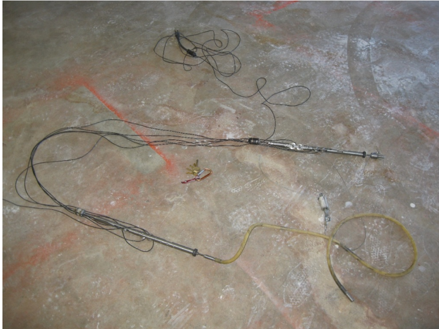
Fig 1. Tether Assembly: stopper → galvanized cable → swivel → upper pulley → lower pulley → hose barb → latex tubing → hose barb → 1/4" all thread (not shown); car keys for scale
