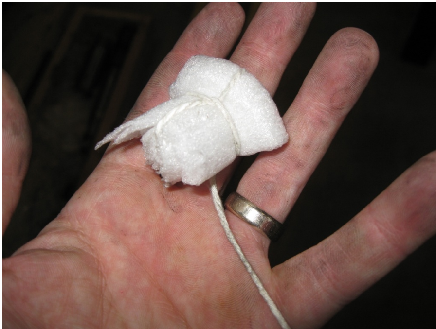
Fig 2. Lightweight string tied around a piece of foam to pass through MDHDS inner barrel assembly using a vacuum or compressed air.
