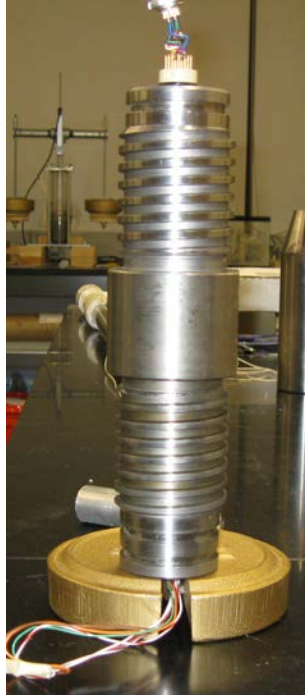
Figure 11: Threaded Union with dangling 15-pin mdm connection
