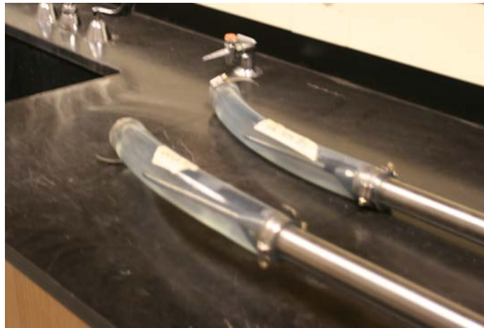
Figure 14: Response chambers with Witness Transducer Port on End
