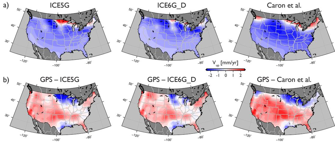
**Figure 5.** a) Vertical rates predicted by ICE-5G (VM2), ICE-6G\_D (VM5a), and Caron et al. (b) Residual velocities after removing model predictions from GPS velocity field.
