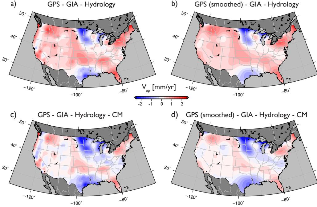
**Figure 7.** (a, d) Residual field after removing, GIA, hydrologic loading, and center of mass translation (CM) from unsmoothed GPS velocity field. (b, c). Same as left, but with smoothed GPS velocity field. Additional intermediate steps can be found in Figure S9.
