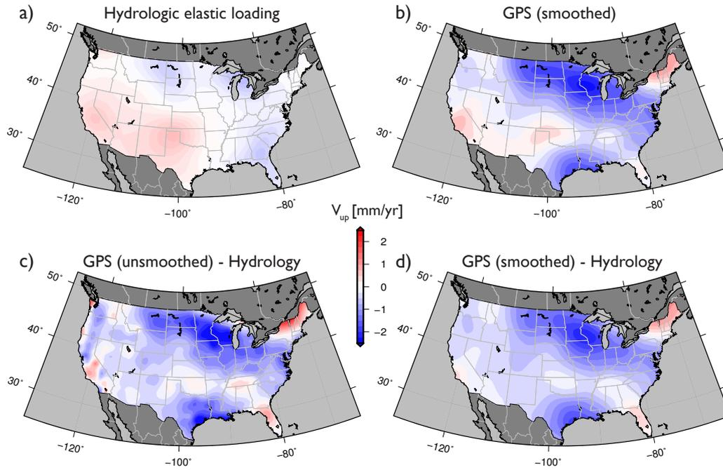
**Figure 6.** (a) Vertical rates due to elastic hydrologic loading, modeled using CSR GRACE-derived terrestrial water storage estimates as input load. (b) 300 km Gaussian smoothed GPS velocity field. (c) Residual velocities after removing hydrologic loading rates from GPS velocity field. (d) Residual velocities after removing hydrologic loading rates from the 300 km Gaussian smoothed GPS velocity field.
