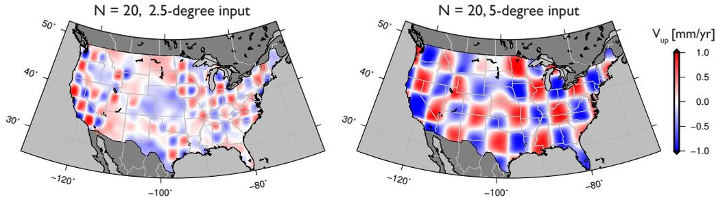
**Figure 2.** Checkerboard test for GPS interpolation resolution using  $N = 20$  centroids, with input checkers of 2.5-degree (left) and 5-degree (right) grids.
